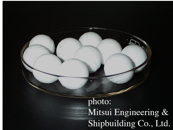
Figure I-11 Photo of natural-gas hydrate pellets (offered by Mitsui Engineering & ShipBuilding, Co., Ltd.).
