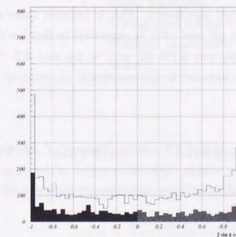
Figure 7.12: The resolution effect causing wrong sign events with M_{ee} < 2 \text{ MeV}/c^2 . The open histogram shows the \sin \phi \cos \phi distribution from the signal Monte Carlo. The hatched and solid histogram indicates the distribution of wrong sign events. The wrong sign events distribute uniformly and it was caused by the X track swapping.
