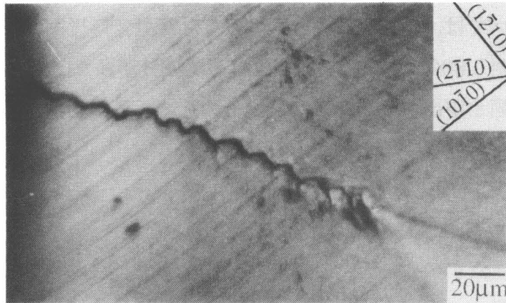
Fig. 4-25 Microcrack path in Ti_3Al single crystal with orientation b cyclically deformed at 800^\circ C and at \Delta\sigma = 100MPa to N=10572 .
