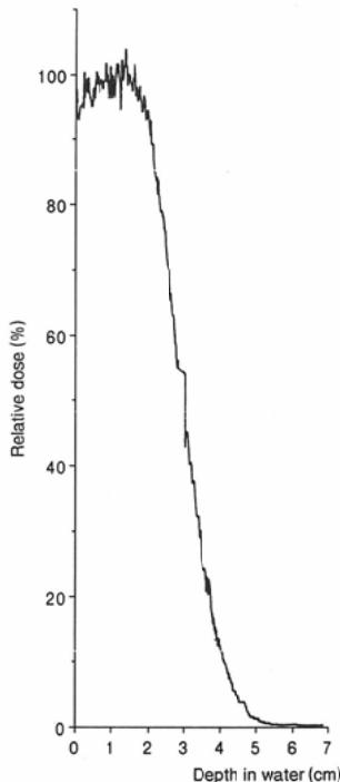
Fig. 2 Depth-dose curve of modulated proton beam with 2cm SOBP in water.
