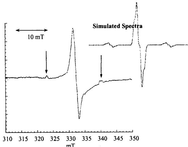
**Figure 3-2-1.** EPR spectrum of defect-containing  $\gamma$ -irradiated PMPS at 6 K with simulated spectrum of  $-\text{MePhSi}-\text{MePhSi}$  using coupling constants in refs. 13 and 15.
