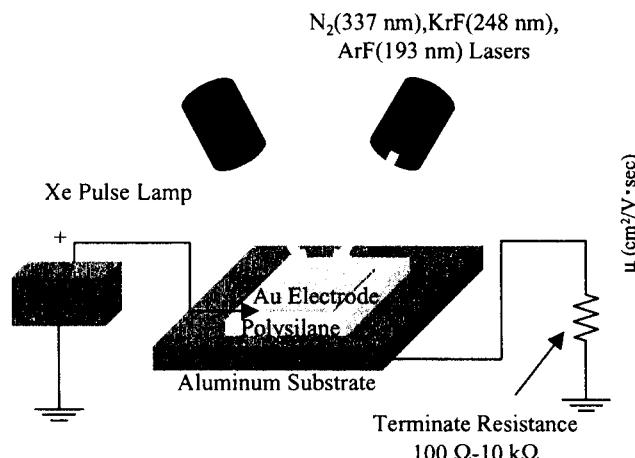
**Figure 3-4-1.** Schematic diagram of the measurement system of TOF.
