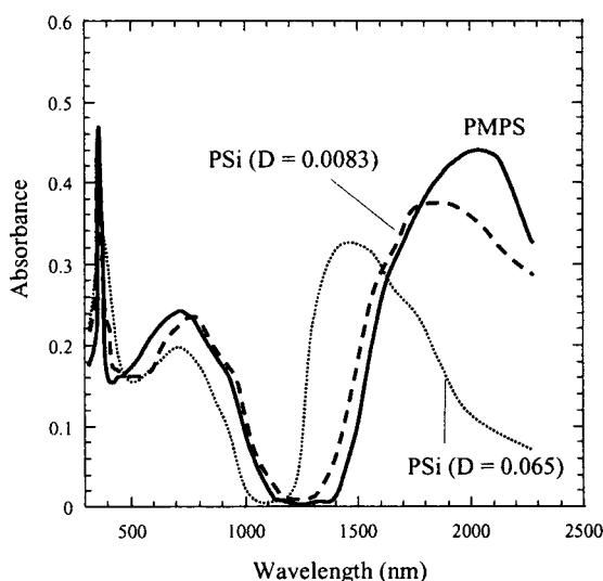
**Figure 3-3-6.** Absorption spectra of polysilanes in MTHF solutions at 77 K. The solutions were irradiated by  $^{60}\text{Co}$   $\gamma$ -rays at 15.7 kGy, and solvated electrons were breached by the exposure to a 527 nm laser light during 1 min. Solid, dashed, and dotted lines indicate the spectra of PMPS, PSi (D = 0.0083), and PSi(D = 0.065), respectively.
