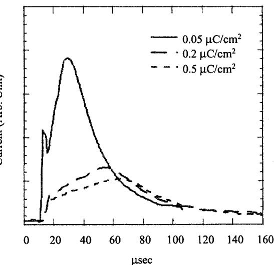
Figure 4-5-3. Changes in transient current pulse shapes of irradiated poly(methylphenylsilane) by 2 MeV H $^+$  ion beam at 298K,  $4.2 \times 10^4 \text{ V}/\text{cm}$
