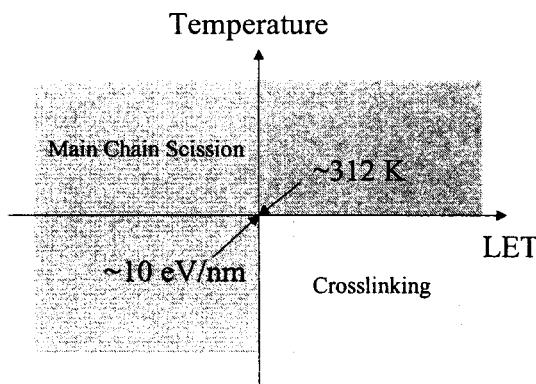
**Figure 4-4-1.** Schematic diagram of predominant reactions in PDHS.
