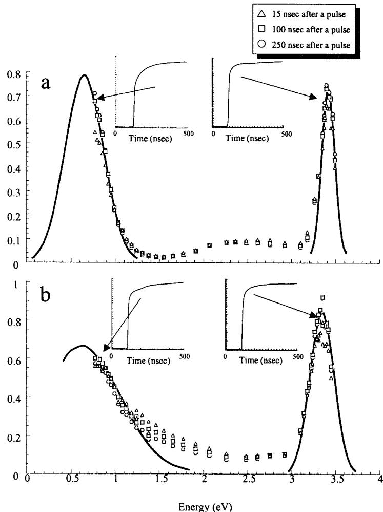
**Figure 3-3-4.** Transient absorption spectra of radical anions : a and radical cations : b of PMPS at the 15, 100, and 250 nsec after a pulse. Superimposed figures indicate the kinetic traces of transient absorption.
