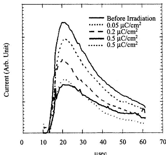
Figure 4-5-4. Changes in transient current pulse shapes of irradiated poly(di-n-hexylsilane) by 2 MeV H $^+$  ion beam at 298K,  $4.2 \times 10^4 \text{ V}/\text{cm}$
