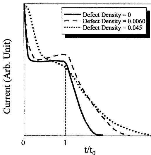
**Figure 3-4-3.** TOF signals measured in PMPS (solid), PSi ( $D = 0.0060$ ) (dashed), and PSi ( $D = 0.045$ ) (dotted) at 295 K,  $E = 6.5 \times 10^5$  V/cm. All curves are normalized at their average flight time.
