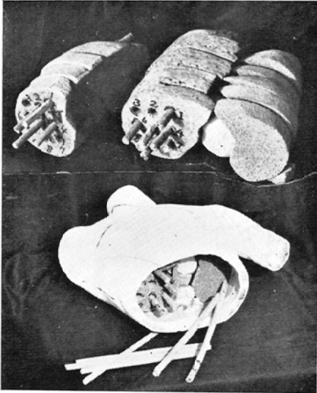
Fig. 3. Chest phantom and lung phantom, lungs are made of cork with two different densities. Nine cork made sticks inserted from the base into the apex of the right lung are made for the insertion of dosimeter.
