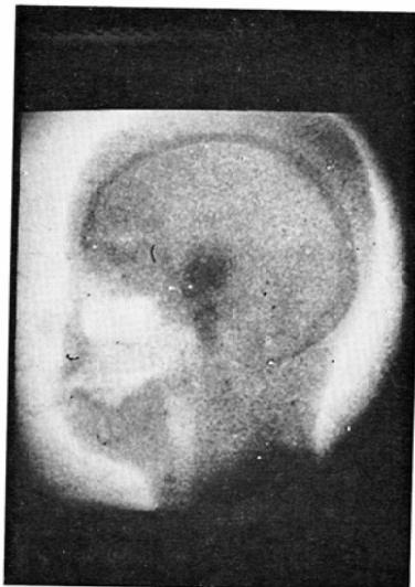
Fig. 11 Fluoroscopy of head phantom, lateral
