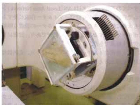
Fig. 2 Setting the 3D compensating filter : The 3D compensating filter was fixed in the gantry.
