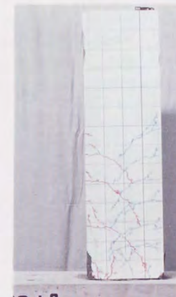
試験体PC-L3 b×D×h0 (mm) ; 400×400×2400 pg=2.15% pg'=0.96% pw=0.60% \sigma_B=323\text{kgf/cm}^2 \sigma_B'=778\text{kgf/cm}^2 N/(bDFc)=0.15 突合せPCa柱
