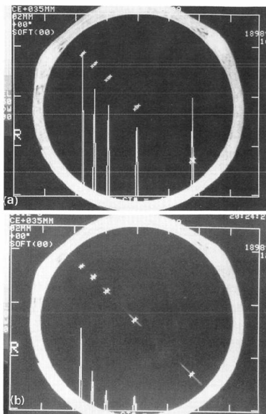
Fig. 5 CT values in profile images: comparison between 1.5mm- and 10mm-thick slices. For visual examination of CT values, profiles perpendicular to the catheters were prepared. In the 10mm-thick slice, the CT value for each catheter is lower, indicating the large influence of the partial volume effect in a thicker slice.
