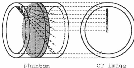
Fig. 2 Schematic presentation of the phantom-simulated broncho-vascular structure and its CT image. Within a plastic cylinder, 6F angiographic catheters are placed in a fan shape (left) and are scanned at slice thicknesses of 1.5mm and 10mm (right).
