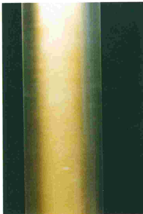
Fig. 7. Thermochromism of 3% polypropylene gel in benzene: colour photographs of scattered light by the gel at (a) 26.6°C; (b) 31.0°C; (c) 36.0°C; and (d) 50.0°C.
