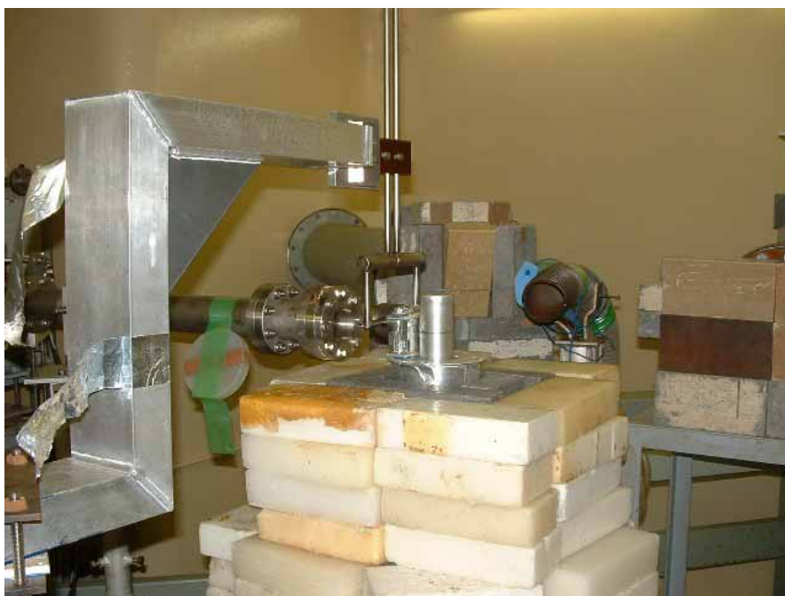
Fig. 5.8: Picture of a whole setup. Beam window, Ta target, tungsten alloy collimator, cryostat, and radiation shield are seen. The sample cell for liquid D_2 was set in the top part of the Al cylinder.
