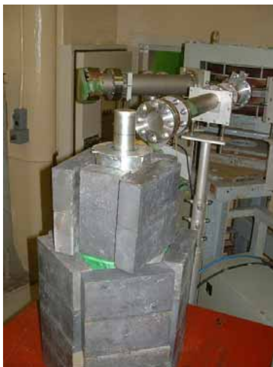
Fig. 5.7: Cryostat shielded by B_4C and lead. In the center of the shield an Al window for the gamma rays is seen. Polyethylene blocks are removed.
