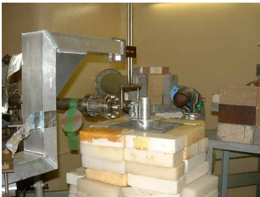
Fig. 5.8: Picture of a whole setup. Beam window, Ta target, tungsten alloy collimator, cryostat, and radiation shield are seen. The sample cell for liquid D 2 was set in the top part of the Al cylinder.
