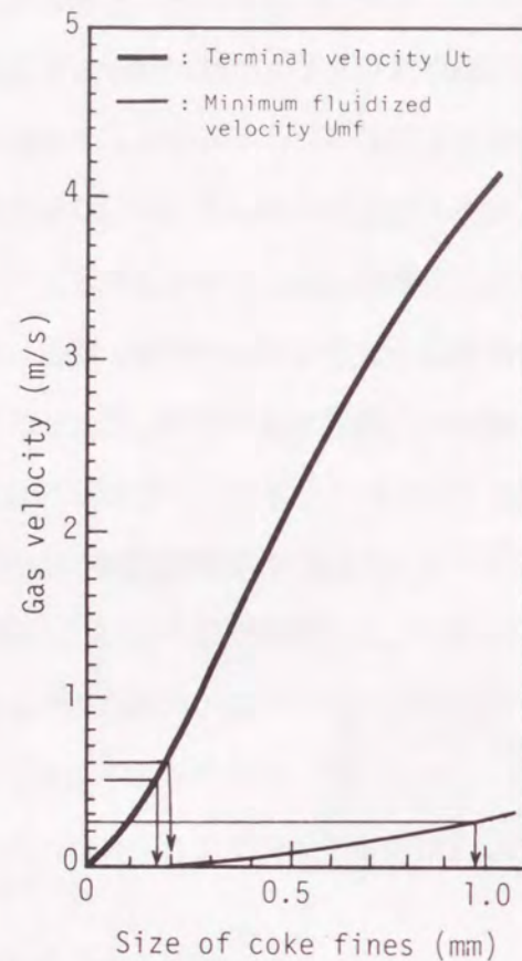
Fig. 6.19 Relationship between size of coke fines and terminal velocity, minimum fluidized velocity.
