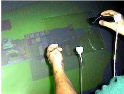
Figure 2.14: The transparent prop consist of a plastic square with a tracking sensor attached to it [Schmalstieg 1999].
