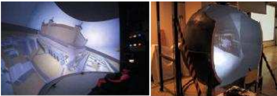
Figure 2.4: On the left, a spherical screen display. On the right, a personal-scale spherical display
