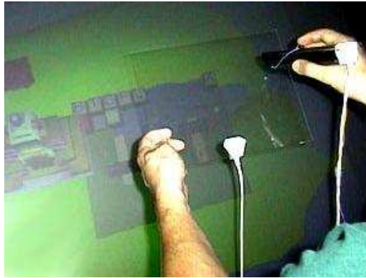
Figure 2.14: The transparent prop consist of a plastic square with a tracking sensor attached to it [Schmalstieg 1999].
