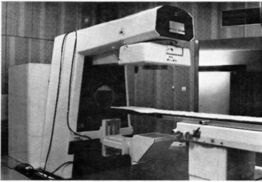
Fig. 2 The field monitoring system fixed on the gantry of 6MV linear accelerator.
