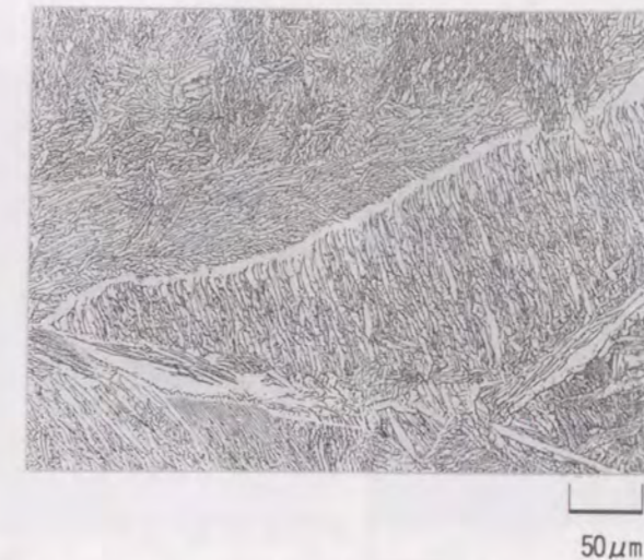
Fig. 6.8 Typical microstructures in the ST6 weld metal.
