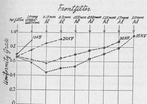
Fig. 8. Uniformity grade at various qualities of soft X-rays.
