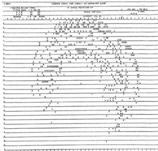
Fig. 19. Computer print-out of the isodose distributions for the tangential rotation calculated by the summation at 6-deg. intervals
