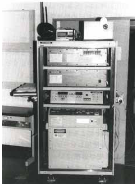
Fig. 2 Apparatus of laser (made by Olympus Optical Co. Ltd.) This is a fun-cooled apparatus. The maximum power is 50W. The output of laser is stable even at low wattage.
