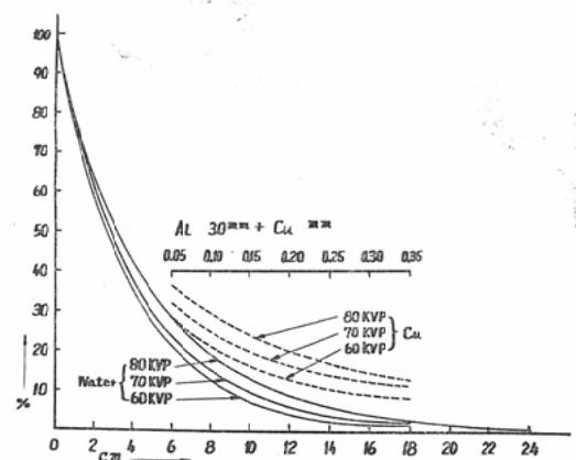
Fig. 4. — : Relationship between thickness of water phantom and dose rate.
