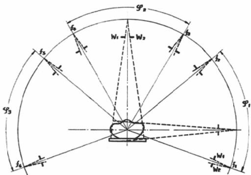
Fig. 1. Mechanism of compensating filter. During the rotation of X-ray tube ( $f$ ) in the range of  $\phi_1$ , the filter works as  $w_1$  and in the range of  $\phi_2$  the filter works as  $w_2$ . These filters absorb the X-ray to the anterior surface of the body, while the X-ray tube rotates in  $\phi_2$ , the filter  $w_1$  and  $w_2$  absorbs the X-ray to the lateral surface.
