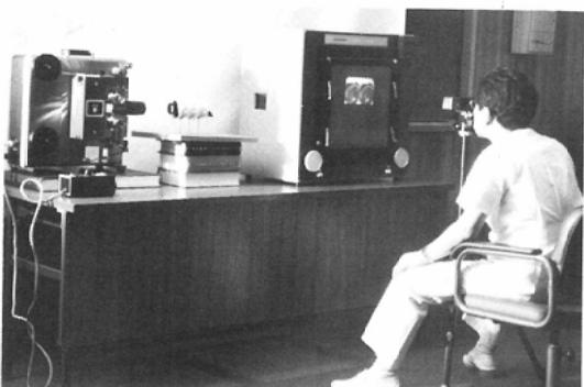
Fig. 5: Two adjacent horizontal pictures are produced by placing a Vanguard XR-35 Prism between the Dynamic Frame 16-B and Screen box. An observer is then able to view the pictures utilizing a stereoviewer.
