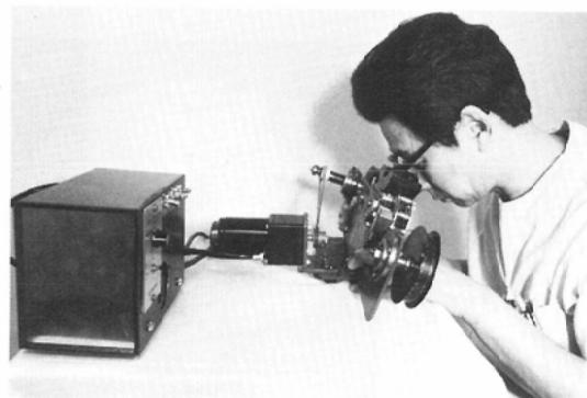
Fig. 4: Electric stereoviewer using Asahi Pentax Stereoviewer Type II
