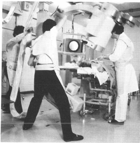
Fig. 8: a) Clinical application showing the need to manually move the C-arm of the CH-41 so as to maintain the "center point" for continuous viewing. This C-arm is equipped with 0.8mm focal spot x-ray tube (Circlex 0.6W/0.8PG 38B) and 9inch image intensifier (Philips 9/5 High Lens) with Arritechno 35R90 using Kodak CFS 35mm cinefilm.
