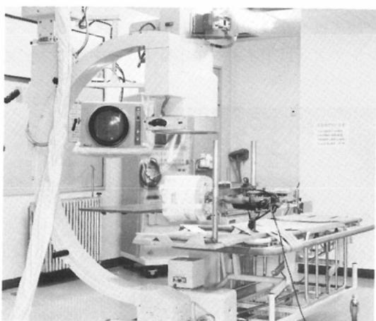
Fig. 2: Rotatostereocineradiography was carried out using a CH-41 and rotating head supporting device occupied a model skull.
