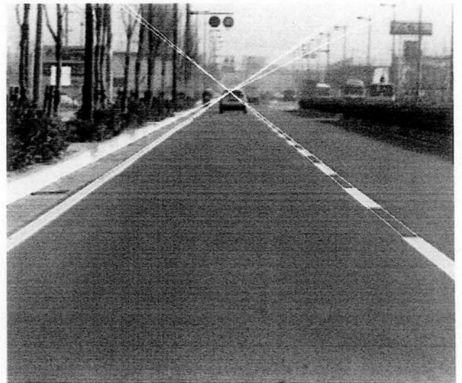
Photo.10.15 Detected lines are Overlaid
