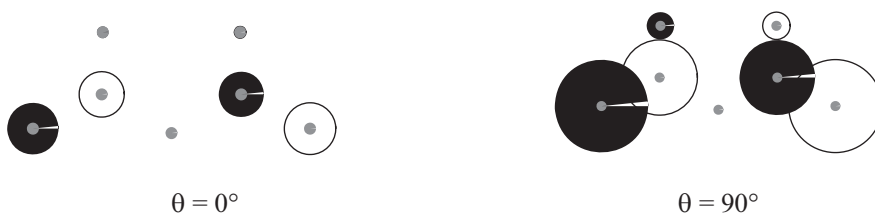
Fig. 7.3. Plots of \gamma_{xxx} densities on the nitronyl nitroxide radical units for the non-(a), donor ( X = \text{NH}_2 )- and acceptor ( X = \text{CN} )-substituted phenyl nitronyl nitroxide radicals, at the rotation angles \theta = 0^\circ and 90^\circ . The dark circle indicates the position of atom.
