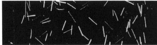
(a) Dilute suspension at a volume fraction of 0.04% ( nL^3 = 0.5 ). Vinylon fibers are clearly visible.
