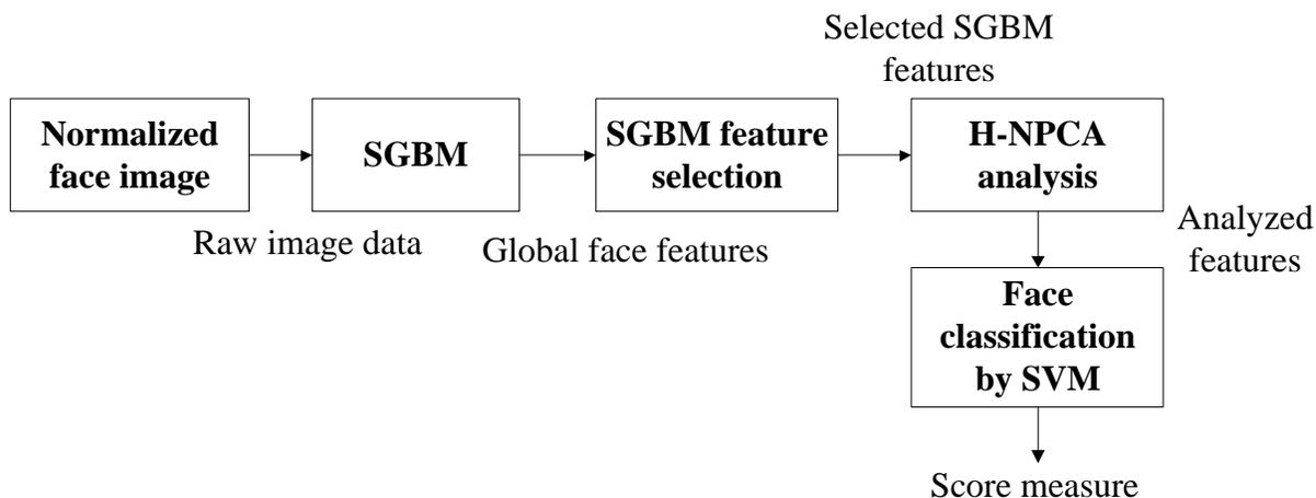
Fig. : Structural diagram of SGBM and H-NPCA
