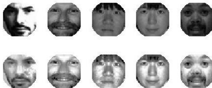
(c) Moustache and beards are also whitened as other parts of the face. The whitening decreases the effect of moustache and beards that significantly improves FAR rates.
