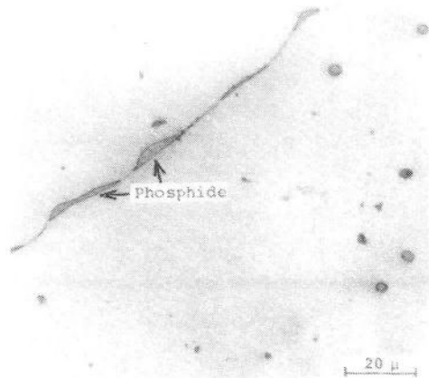
Photo.4.1 Microstructure of SUS 304-P3 weld metal containing about 0.24%P, showing film-like phosphides along columnar grain boundary.
