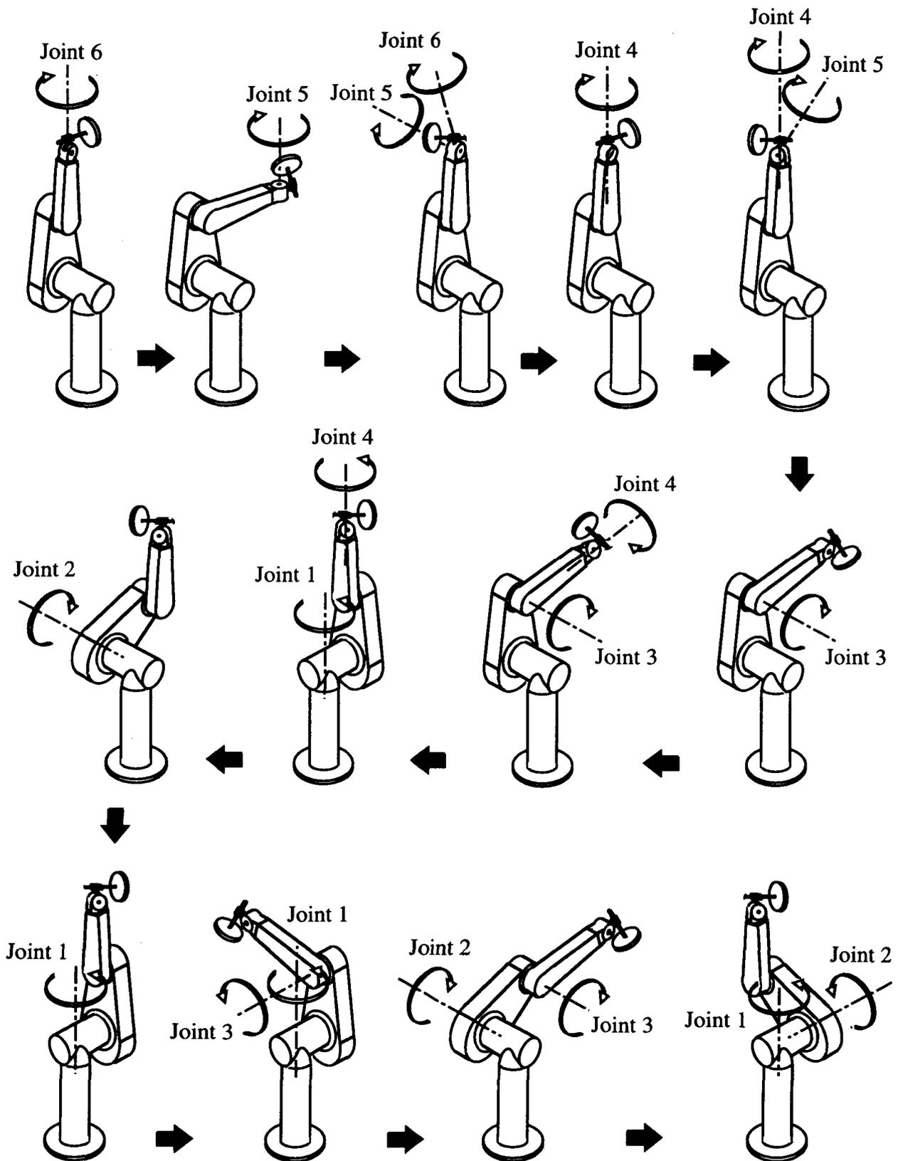
Fig. 3.4.1 The Accelerated Motion Tests for PUMA 560
