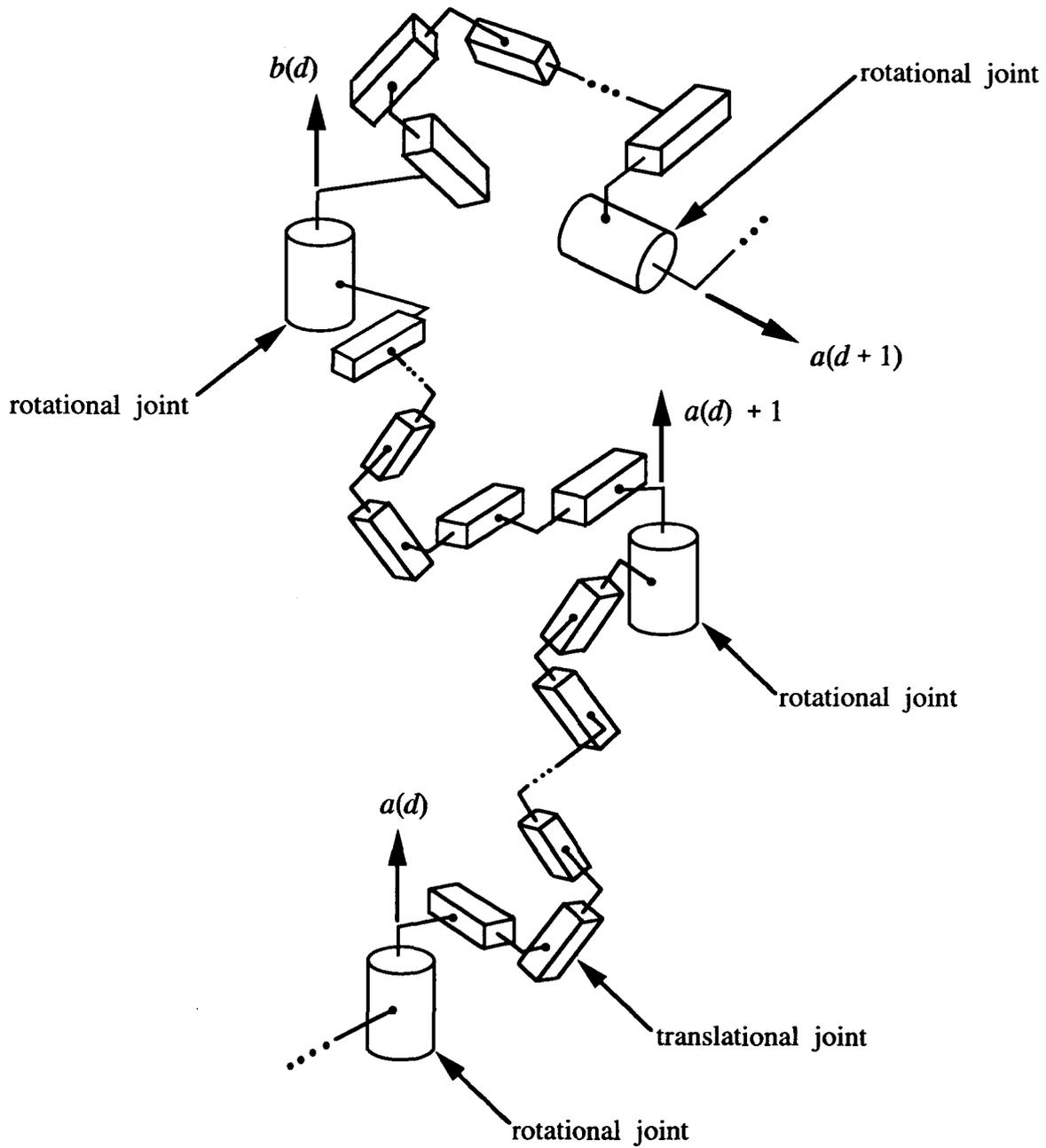
Fig. 2.4.2 d-th Link Cluster in the Manipulator
