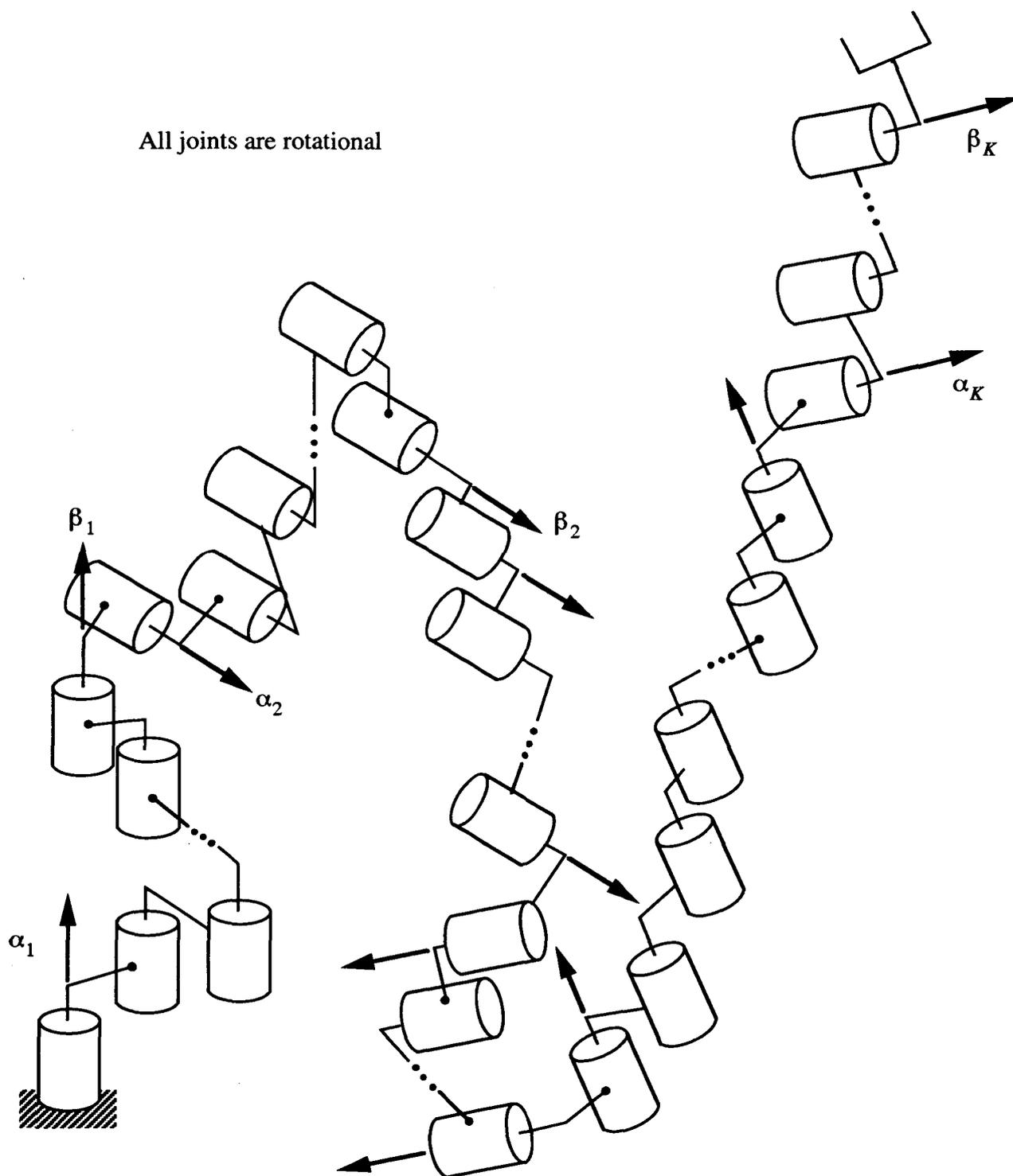
Fig. 2.3.2 Link Clusters in Parallel and Perpendicular Manipulator
