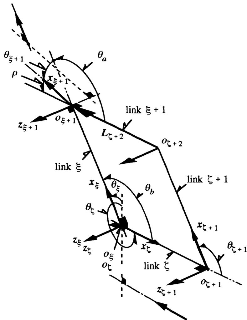
Fig. 2.5.2 Schematic Diagram of the Planar Parallelogram
