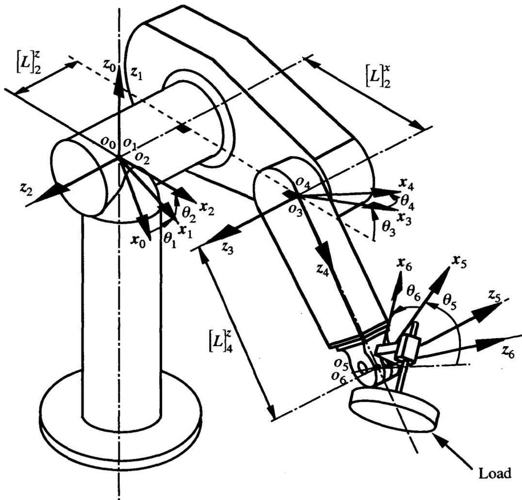
Fig. 3.2.1 PUMA 560 with Load and Its Coordinate Systems
