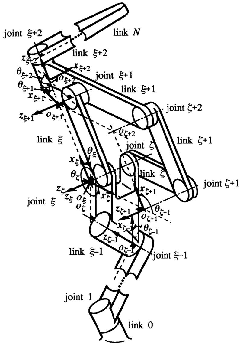
Fig. 2.5.1 Manipulator with a Planar Parallelogram Link Mechanism
