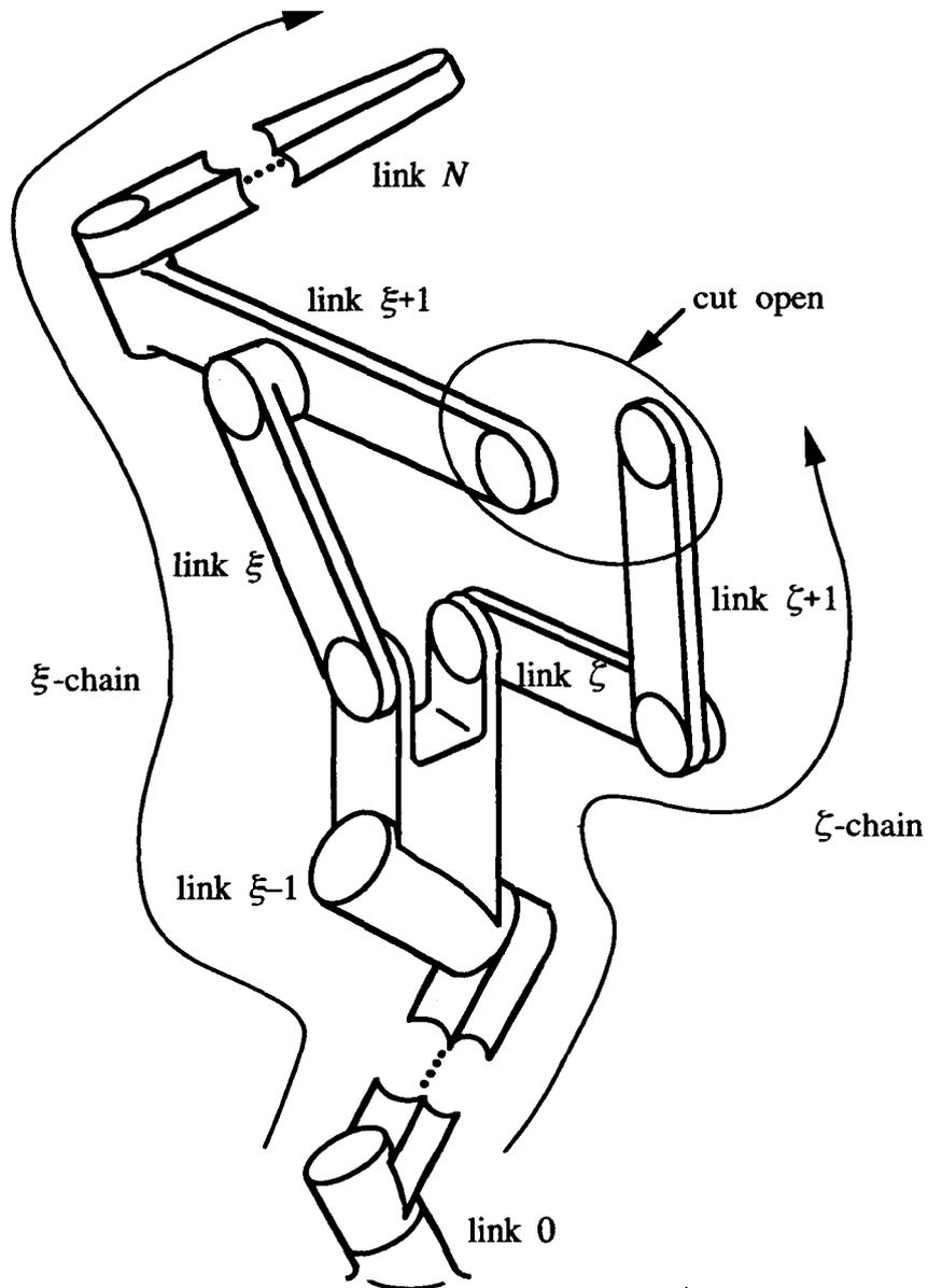
Fig. 2.5.3 Tree Structured Manipulator
