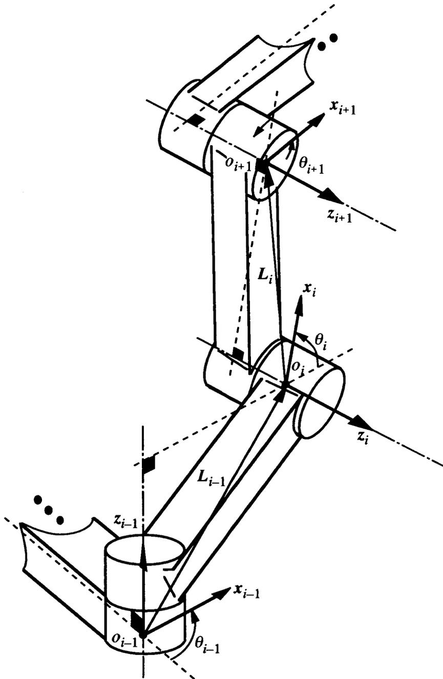
Fig. 2.3.1 Parallel and Perpendicular Manipulator and its Coordinate Systems
