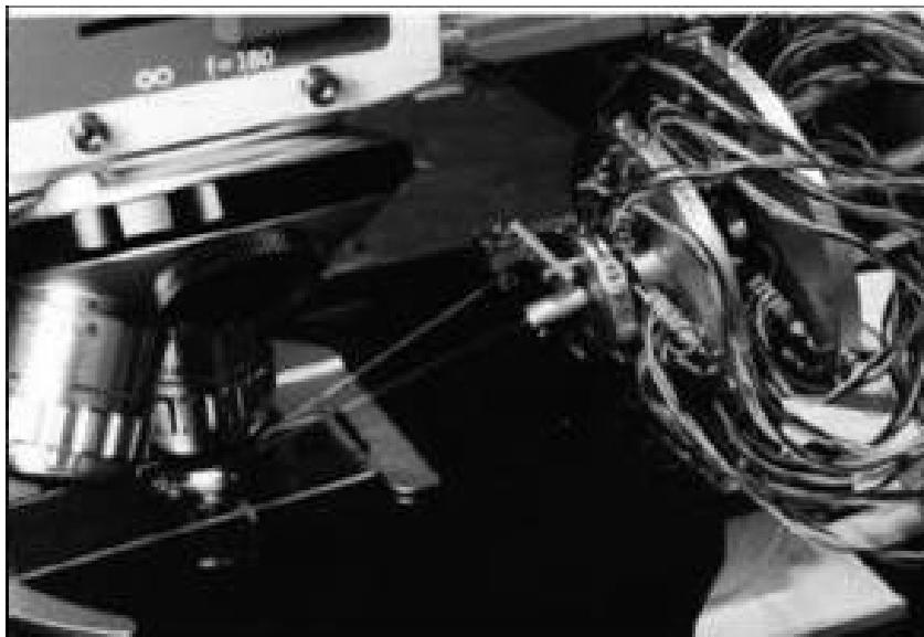
Fig. 1.5: Two-fingered micro manipulator, old prototype 1996.
