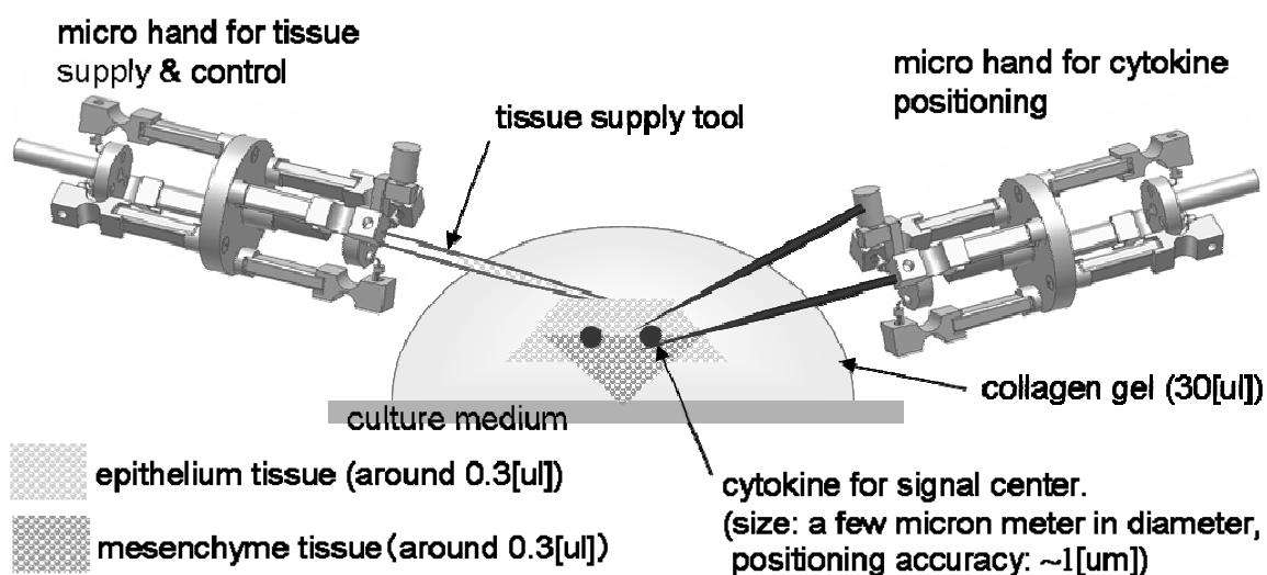
Fig. 4.19: Proposed setup of tissue micro-injection experiment
