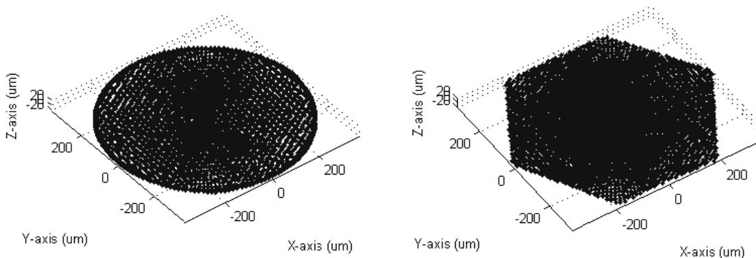
Fig. 3.14: Workspace of 3-DOF PRS micro finger module: Genetically optimized (left) and discrete search method optimized (right)
