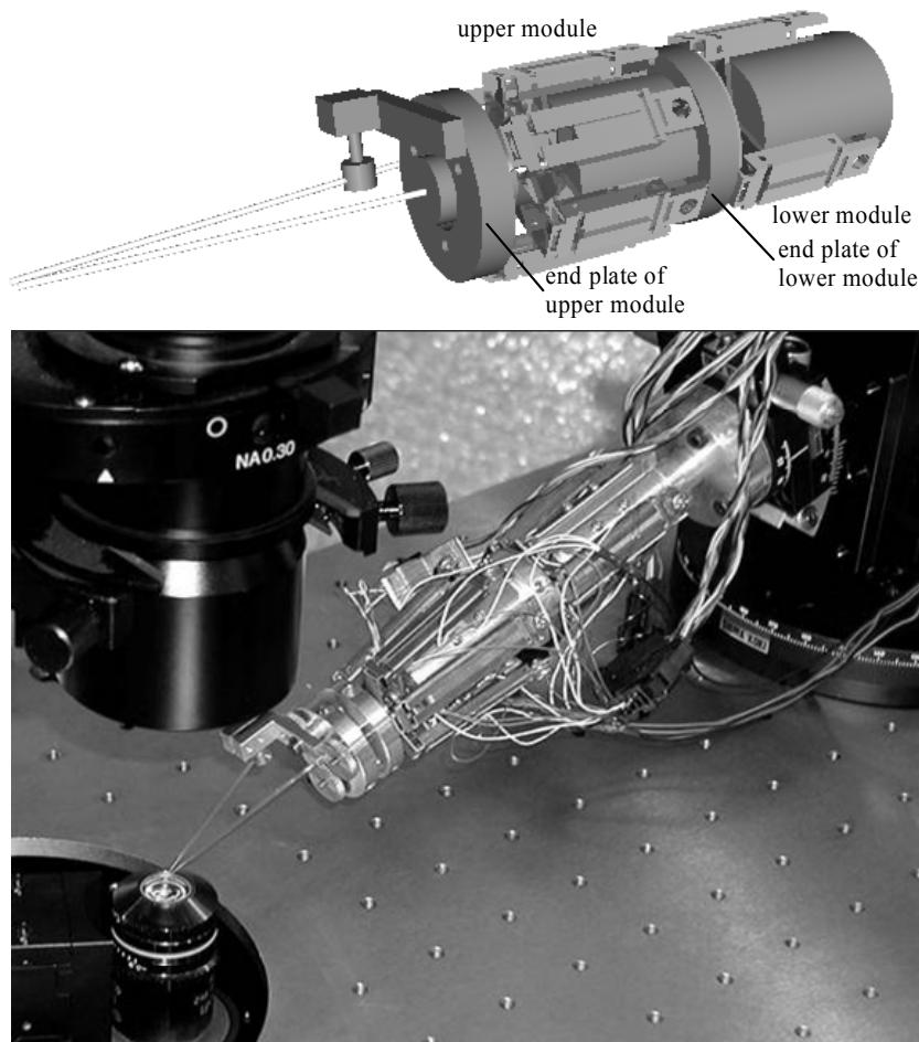
Fig. 4.3: Old prototype of two-fingered micro mechanism with thin plate.
