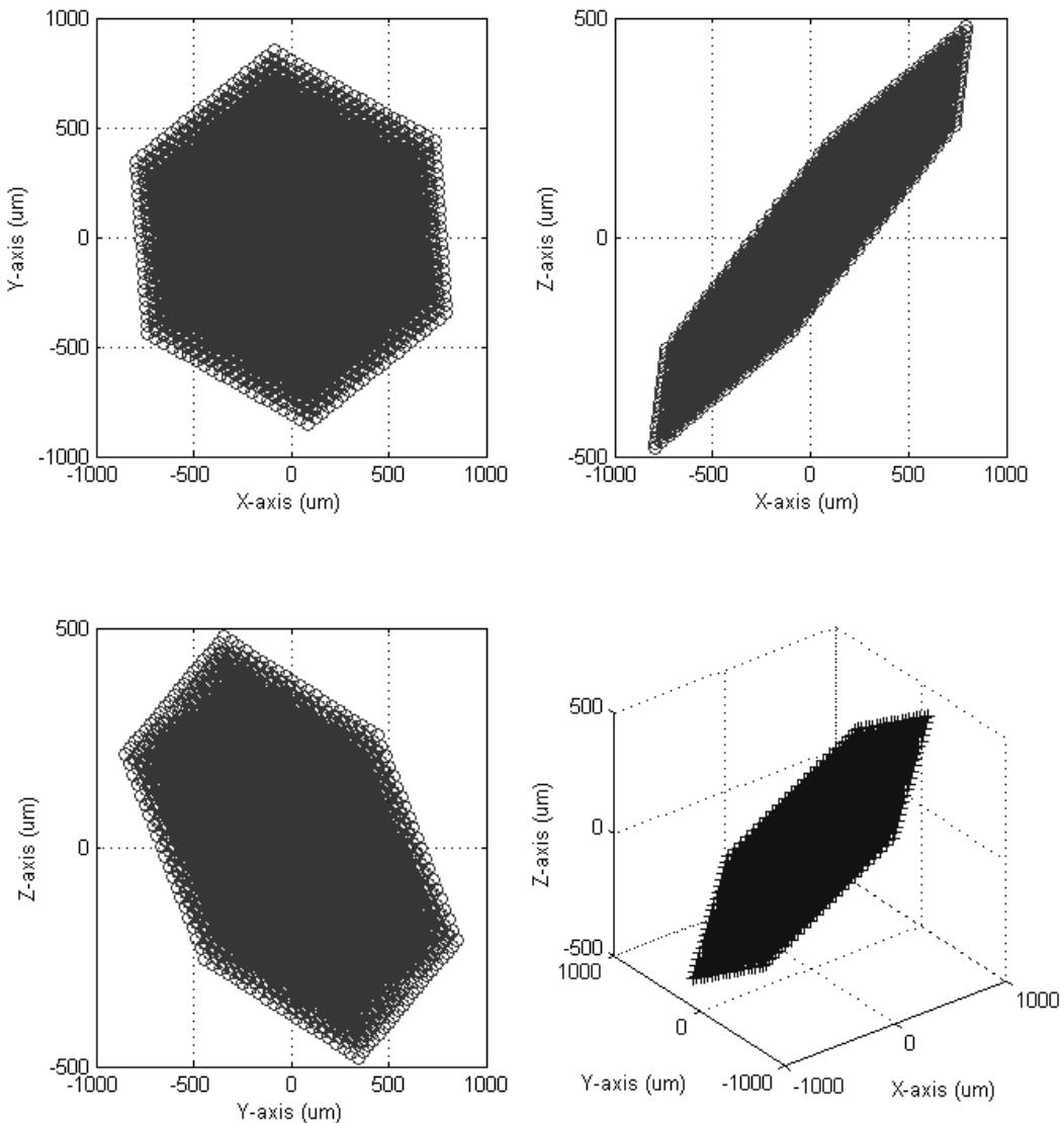
Fig. 4.16: Practical workspace volume of lower finger tip
