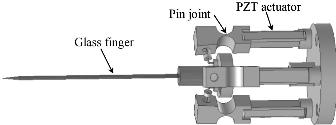
Fig. 3.19: 3-DOF PRS micro finger CAD model
