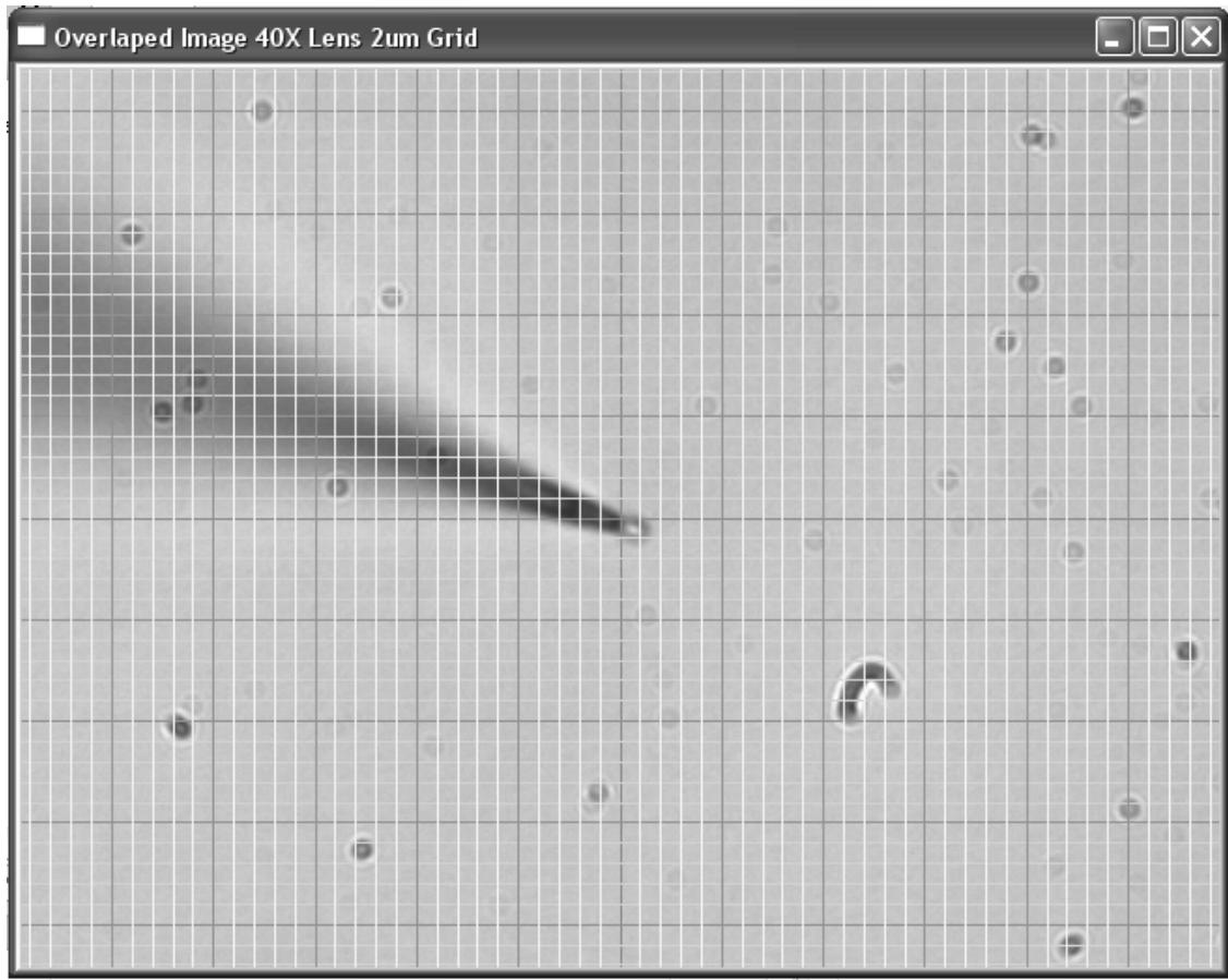
Fig. 4.14: On screen scale for determining XY-coordinates
