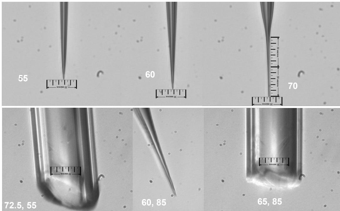
Fig. 4.21: Sample tips produced by PC-10 puller
