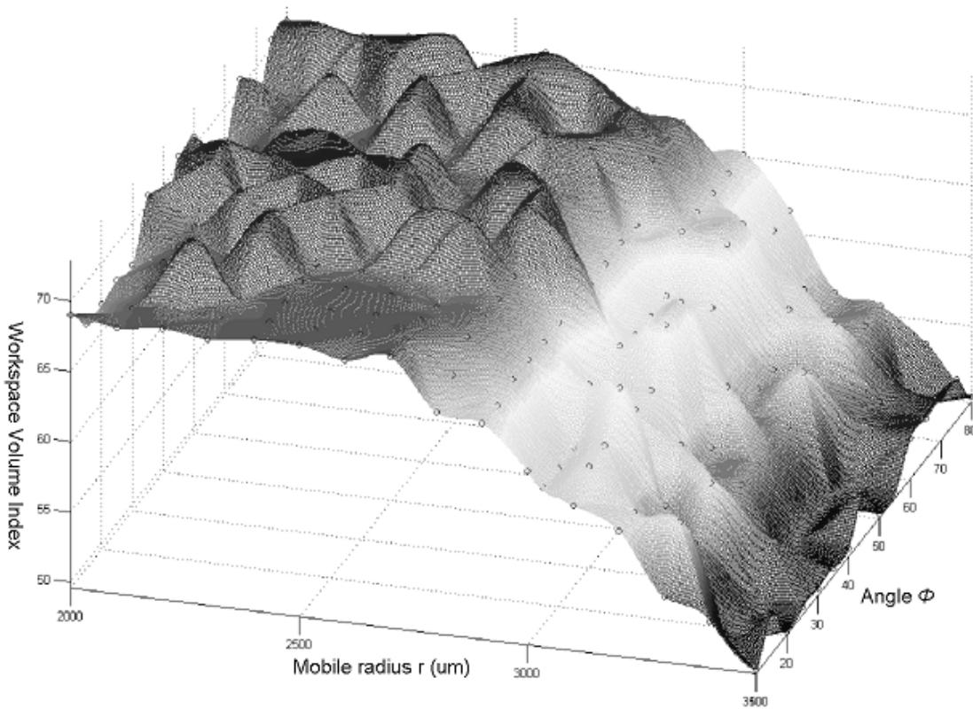
Fig. 3.15: Workspace volume index surface variation vs.  $r$  and  $\varphi$  parameters.  $R=8\text{mm}$
