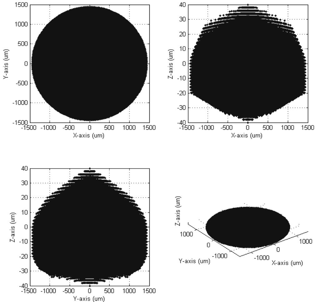
Fig. 3.13: GEAs method: workspace volume of Upper finger tip
