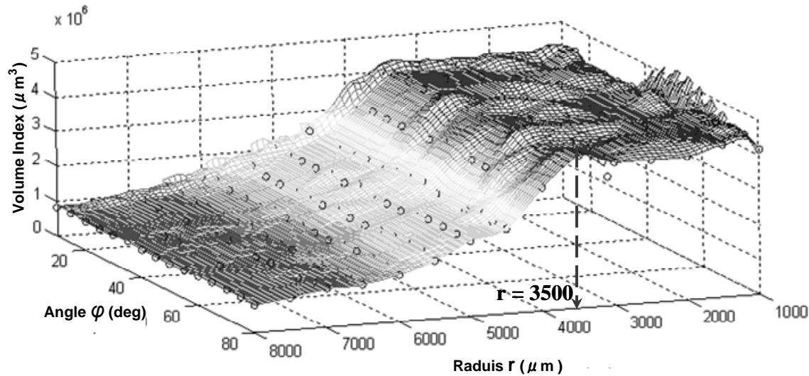
Fig. 3.5: Volume index surface variation vs.  $r$  and  $\varphi$  parameters.  $R=10\text{mm}$
