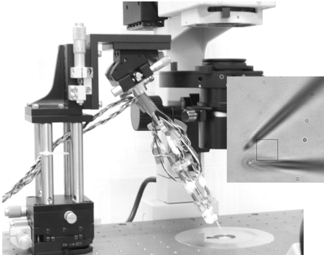
Fig. 4.11: Setup of the two-fingered micro-manipulator hybrid hand
