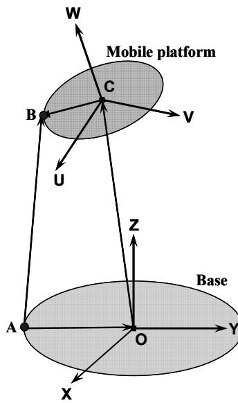
Fig. 2.3: Position vectors of the connecting points of the linking leg.
