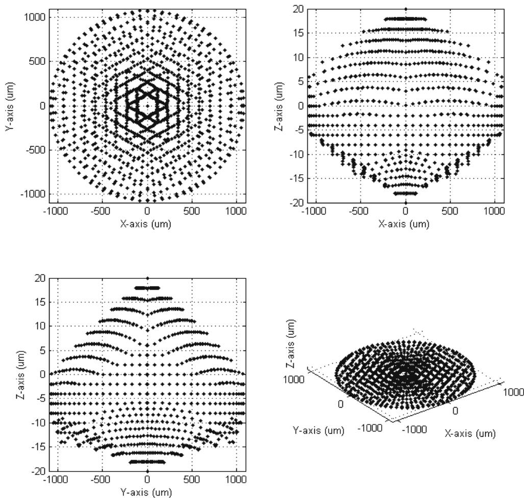
Fig. 3.11: GEAs method: workspace volume of lower finger tip
