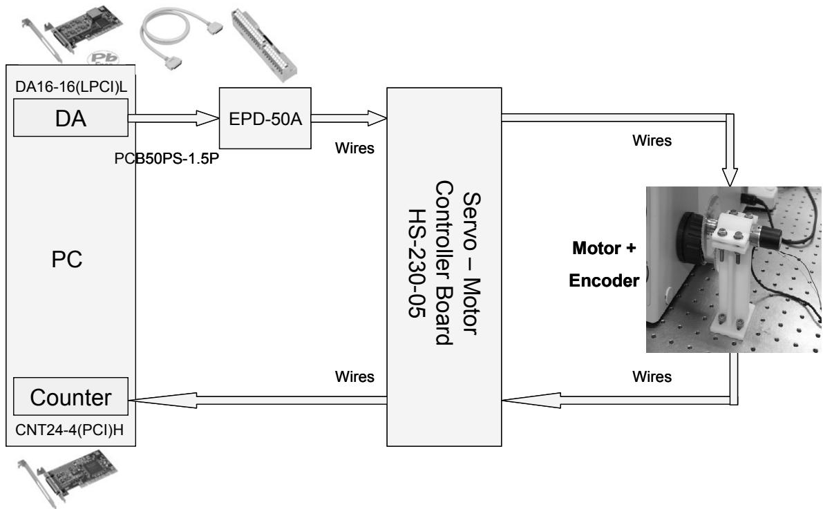
Fig. 4.6: Details of hardware system setup for image processing loop.
