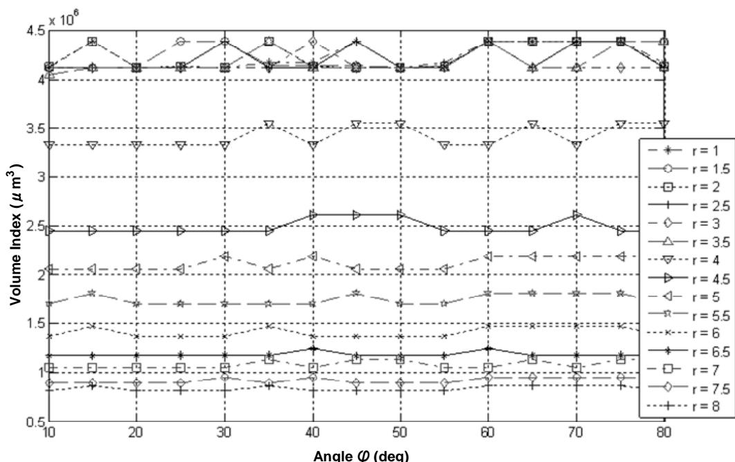
Fig. 3.6: Workspace volume variation vs.  $\varphi$  for different values of mobile radius  $r$ .  $R=10\text{mm}$
