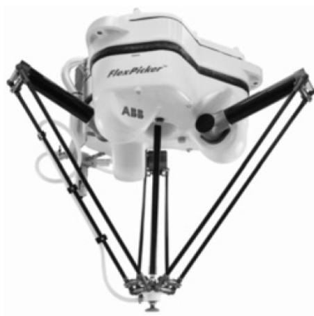
Fig. 1.2: Example of parallel manipulator
