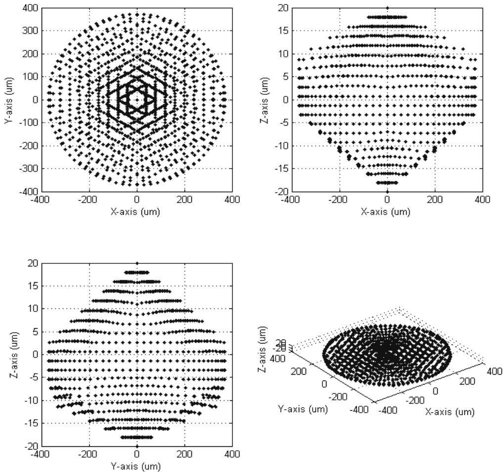
Fig. 3.12: GEAs method: workspace volume of Upper finger tip
