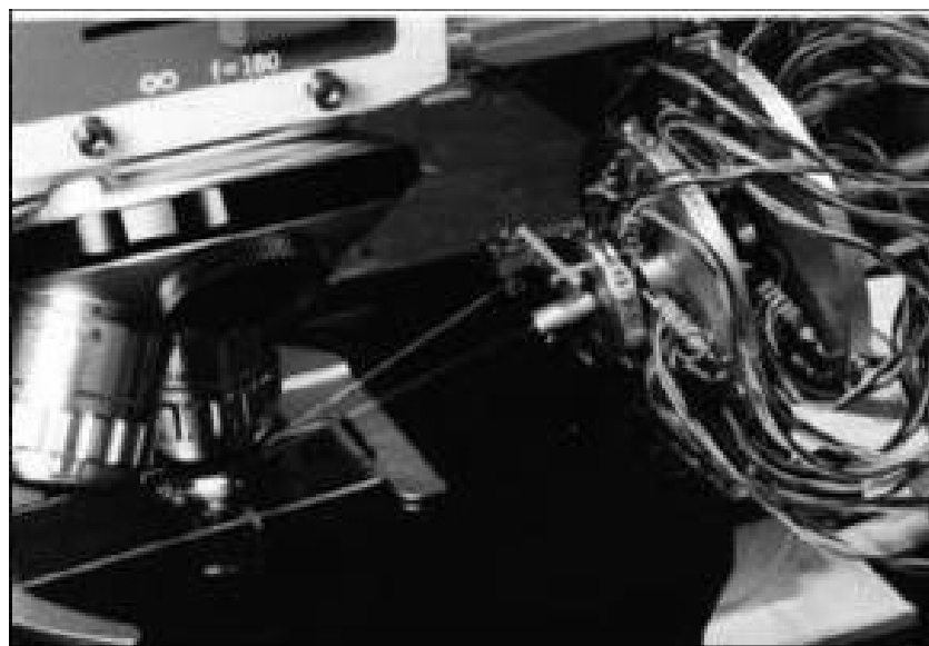
Fig. 1.5: Two-fingered micro manipulator, old prototype 1996.
