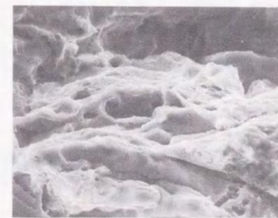
(b) Irregular fracture (localized high plastic deformation)
