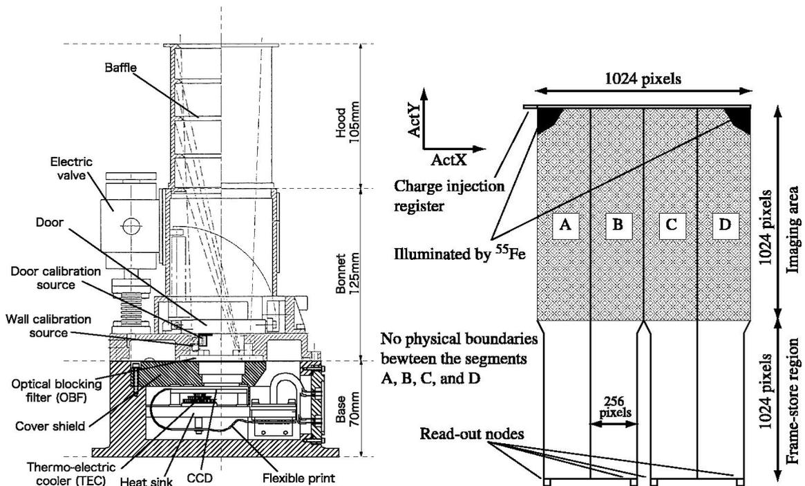
Figure 3.5: Schematic views of *Suzaku* XIS system (left) and XIS CCD (right) (Koyama et al. 2007).
