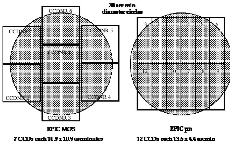
Figure 3.2: Schematic views of the FOV of the EPIC cameras; MOS (*left*) and pn (*right*). The shaded circle depicts a 30' diameter area.
