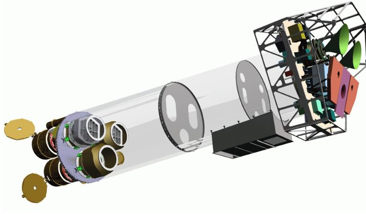
Figure 3.1: Sketch of the *XMM-Newton* observatory. To the left the three mirror modules (with the Reflection Grating Arrays units mounted behind two of them) can be seen, while at the right the back-end of the instrument platform with all the radiators is visible; the EPIC-MOS cameras with their radiators in green, the radiator of the EPIC-pn camera in violet, and the RGS detectors in orange (Jansen et al. 2001).
