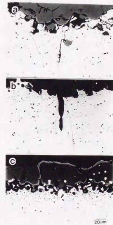
Fig. 3-7 Effect of Mn on the primary scale/steel interface of 0.1%Si-0.020%Ni steels after oxidation at 1220°C for 2h in 77.1%N<sub>2</sub> + 14.3%H<sub>2</sub>O + 8.6%CO<sub>2</sub>.
