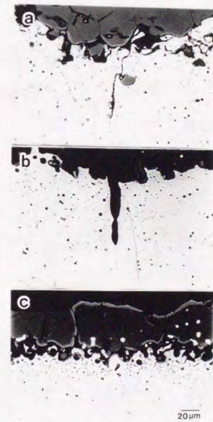
Fig. 3-7 Effect of Mn on the primary scale/steel interface of 0.1%Si-0.020%Ni steels after oxidation at 1220°C for 2h in 77.1%N 2 + 14.3%H 2 O + 8.6%CO 2 .
