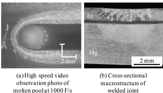
Fig. 2 Welding phenomenon during *heat-conduction* mode welding, and cross section of lap-welded joint between Zn-coated SP781 steel and AZ31B alloy.
