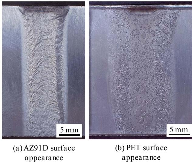
Fig. 4 Surface appearances of *heat-conduction* welded joint between AZ91D and PET.
