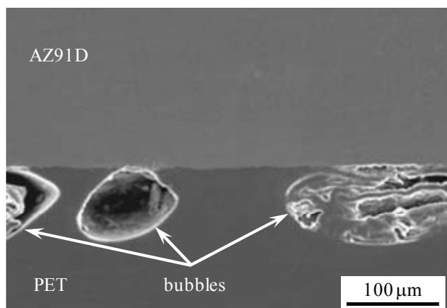
Fig. 5 SEM photo near AZ91D-PET joint interface showing the existence of bubbles in PET and tight bonding between alloy and plastic.
