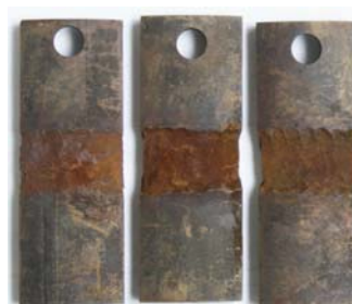
Fig.6 Changing of specimen in corrosion experiment
