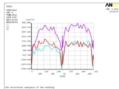
Fig.9 distribution of residual stress on the seam between exosphere and assistance plate(path 4)
