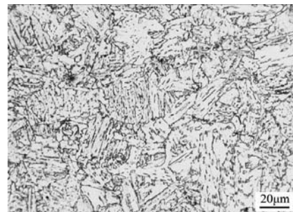
(a) Ordinary X80 pipeline steel
