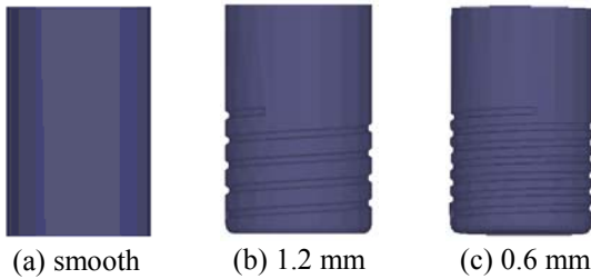
Fig.3 The model of fluid flow simulation and stir-pin
