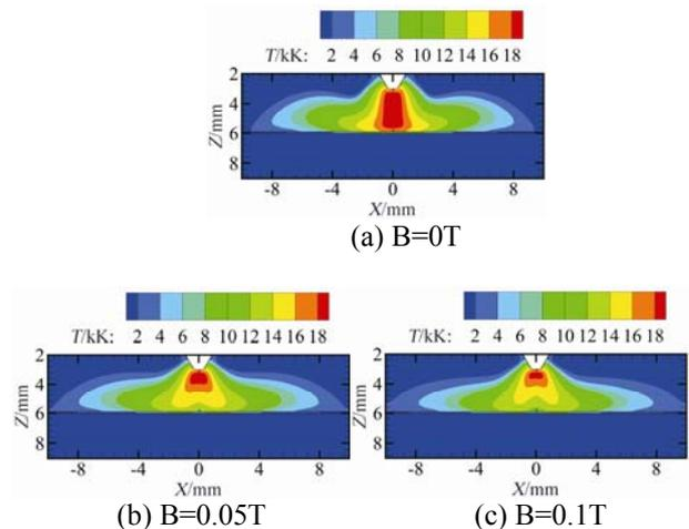
Fig.6 Temperature distribution in the axial section
