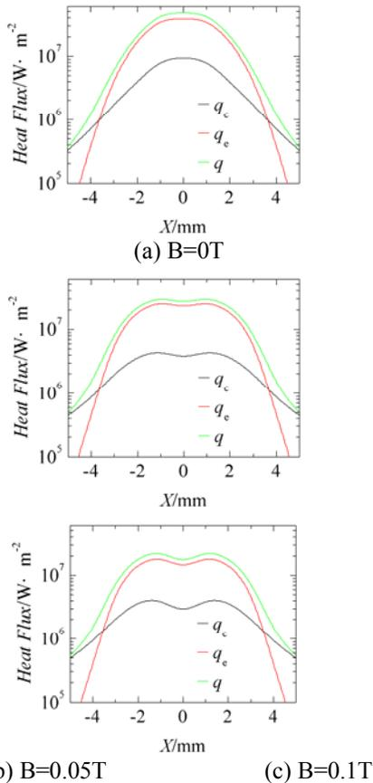
Fig7. Heat flux of arc at anode surface
