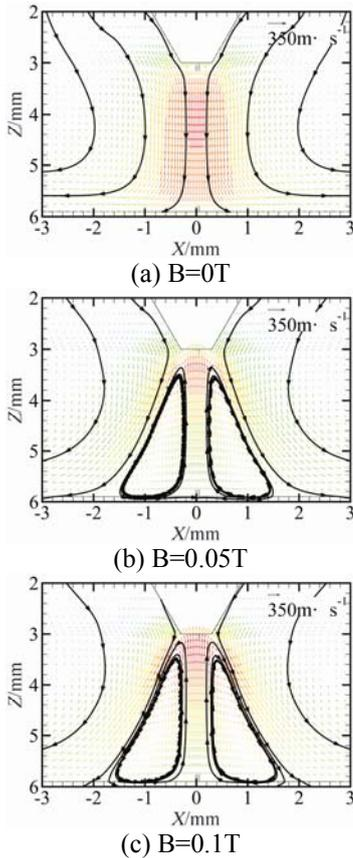
Fig. 4 Velocity distribution of arc in axial section
