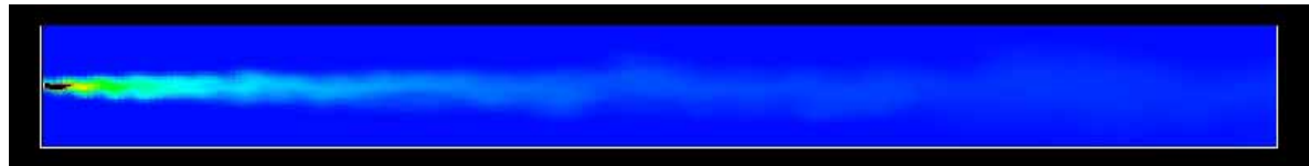
Fig. 7.9: Comparison of instantaneous contours of f_L k_{SGS} among LES with and without PDF model, at T = 32 , z/H = 0.483 .
