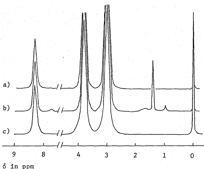
Figure II-23. ^1\text{H} NMR spectra for poly( \beta -alanine) from the polycondensation of 5g in diethyl ether at 30^\circ\text{C} (measured in trifluoroacetic acid).
