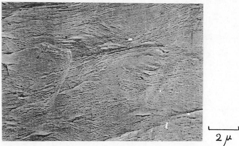
(a) \sigma = 29 \text{ Kg/mm}^2 , N = 2 \times 10^4
