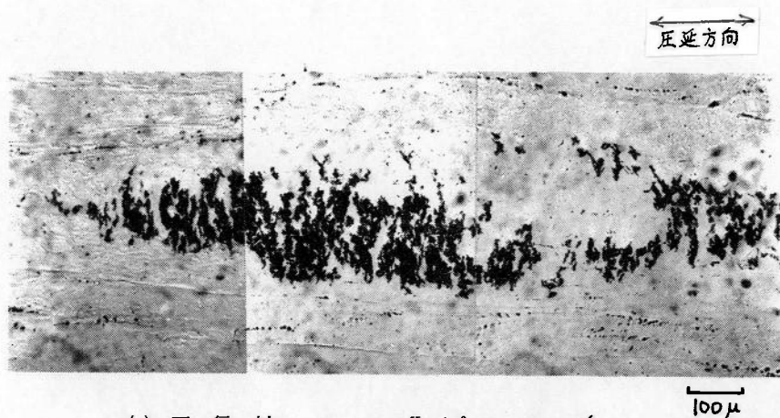
(a) 平行材 \sigma = 19.5 \text{ Kg/mm}^2 , N = 2 \times 10^6
