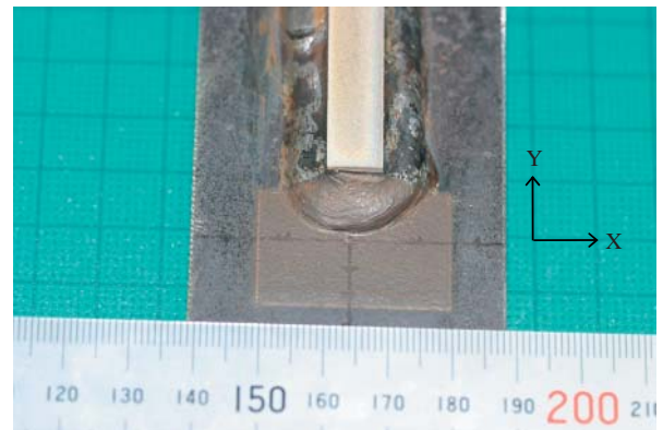
Fig. 3 Laser peened toe of box welded joint
