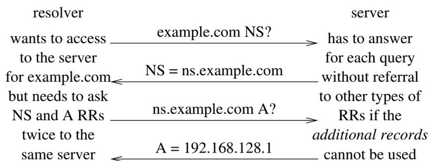
Figure 2.6 DNS name resolution without additional records
