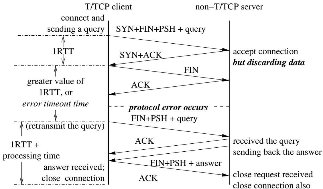
Figure 4.3 Time line of T/TCP client and non-T/TCP server on FreeBSD 4.6.2-RELEASE
