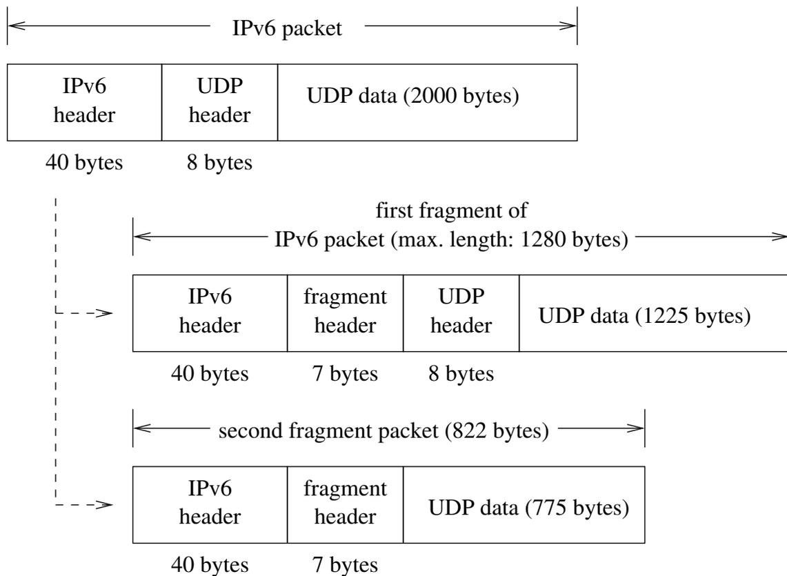
Figure 3.11 An example of IPv6 UDP fragmentation
