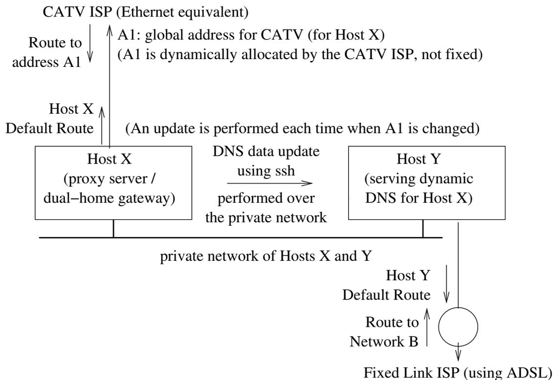
Figure 2.13 An example of dynamic DNS update using ssh
