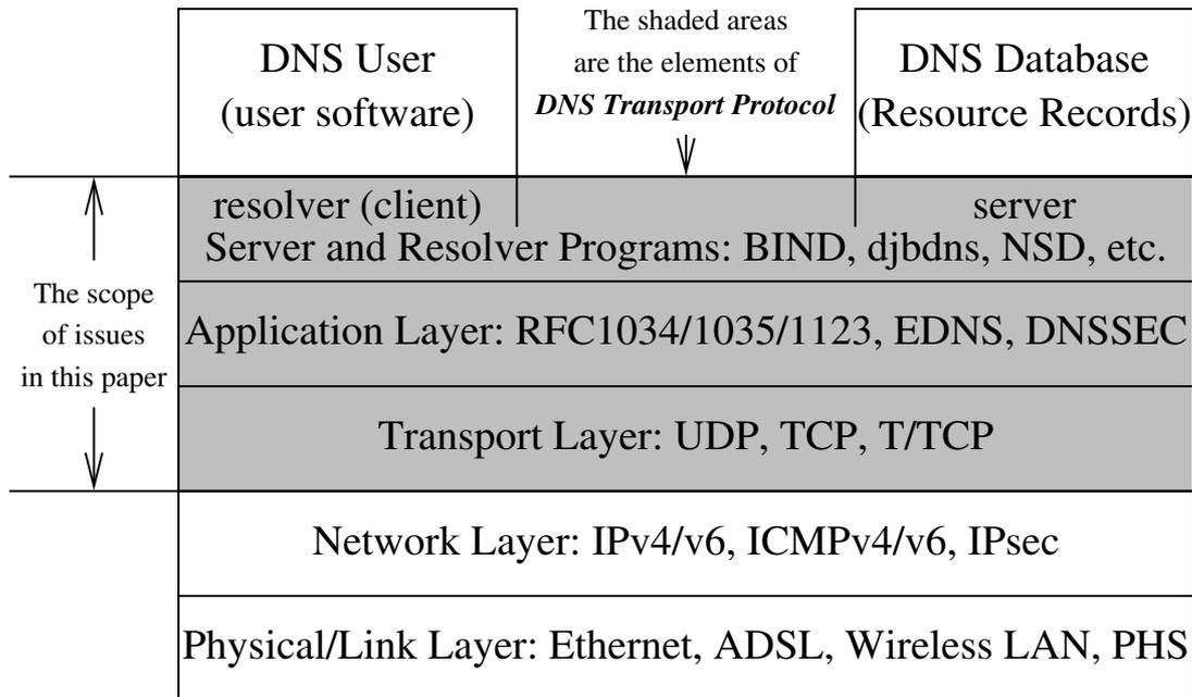
Figure 2.1 DNS protocol layers and the elements
