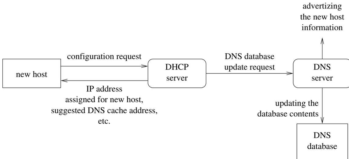
Figure 2.11 Updating DNS database from DHCP server
