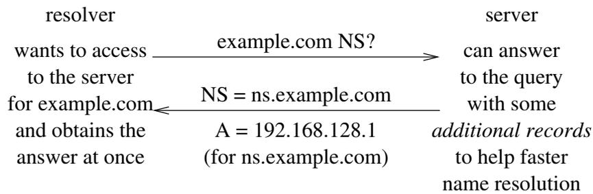
Figure 2.7 DNS name resolution *with* additional records
