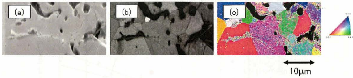
Fig. 2.38 The crack generating from the vertex of the Vickers impression of UN
