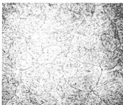
(a) Prior austenite grain size : 0.05 mm
