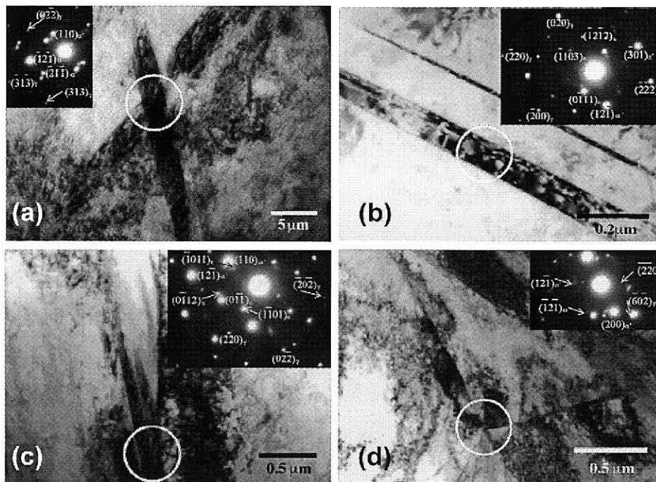
Fig. 1-3 Nucleation sites of  $\alpha'$ -martensite in austenite stainless steel: intersection of  $\epsilon'$ -martensites (a), isolated  $\epsilon'$ -martensite (b),  $\epsilon'$ -martensite-grainboundary (c) and grain boundary triple point (d), respectively. (after Das *et al.* [30])
