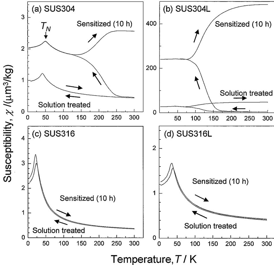
Fig. 2-1 (a-d) Magnetic susceptibility of solution-treated and sensitized stainless steels. Measurement was made in the cooling process and then in the heating process.
