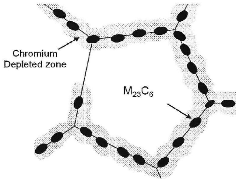
Fig. 1-7 Schematic diagram of carbide precipitation formed along the grain boundaries.
