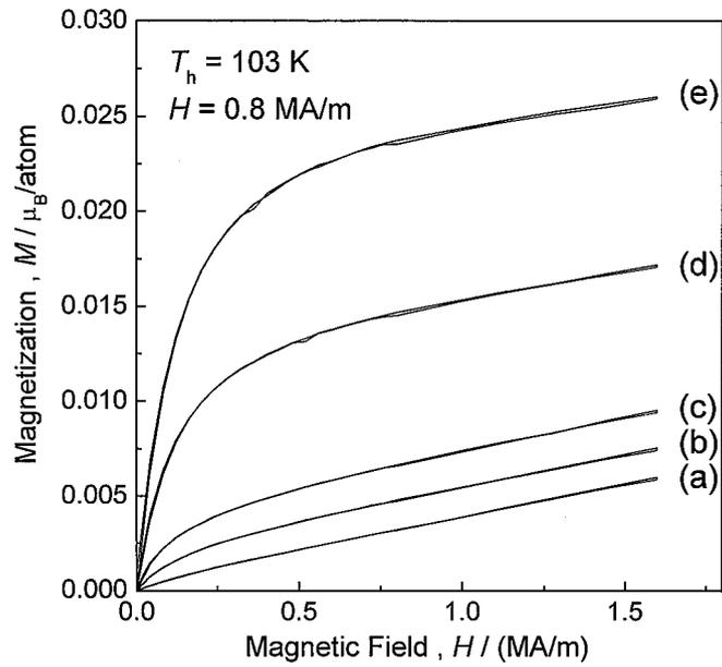
Fig. 5-1 Magnetization curves obtained at 300 K for the solution-treated SUS304L stainless steel after isothermal holding at 103 K for 70 s (a), 210 s (b), 760 s (c), 1680 s (d) and 4860 s (e), respectively, under magnetic field of 0.8 MA/m.
