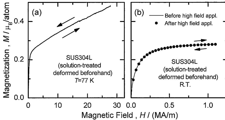
Fig. 2-11 Magnetization curve at 77 K of a solution-treated SUS304L stainless steel under a pulsed high magnetic field (a), and magnetization curve at room temperature in a low field region before and after the high field application (b). Prior to high field application, the specimen was worked by 5% at 77 K.
