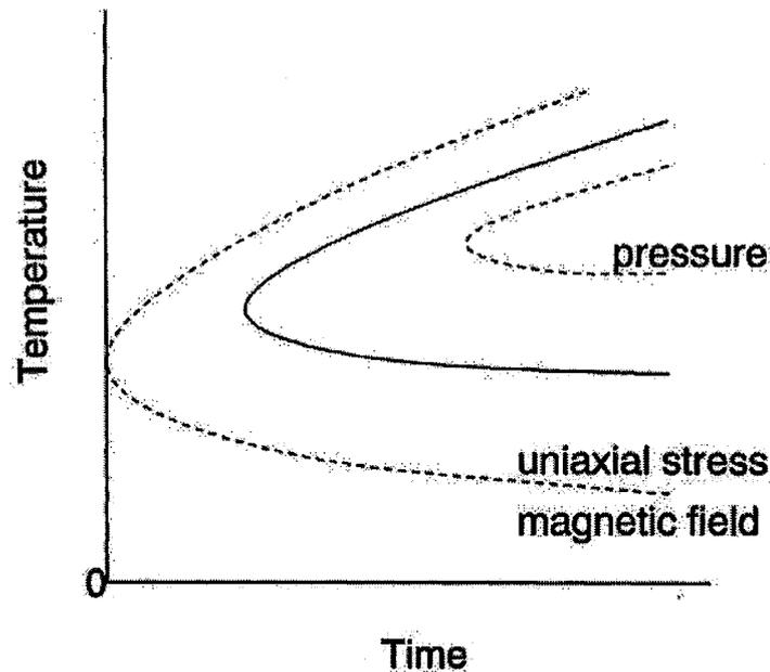
Fig. 1-6 Predicted *TTT* diagrams of isothermal martensitic transformation under magnetic field and hydrostatic pressure by the theory previously constructed, together with that under no external field. (after Kakeshita *et al.* [47])
