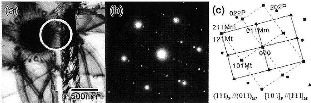
Fig. 2-6 A transmission electron micrograph showing  $\alpha'$  martensite formed in a sensitized (100 h) SUS304 stainless steel (a), the diffraction pattern taken from encircled area (b) and its schematic illustration (c). The diffraction pattern includes reflections from  $\gamma$ -phase (P), matrix of  $\alpha'$  martensite (Mm) and its twin (Mt). The  $\gamma$ -phase and  $\alpha'$ -martensite satisfy the K-S relation.
