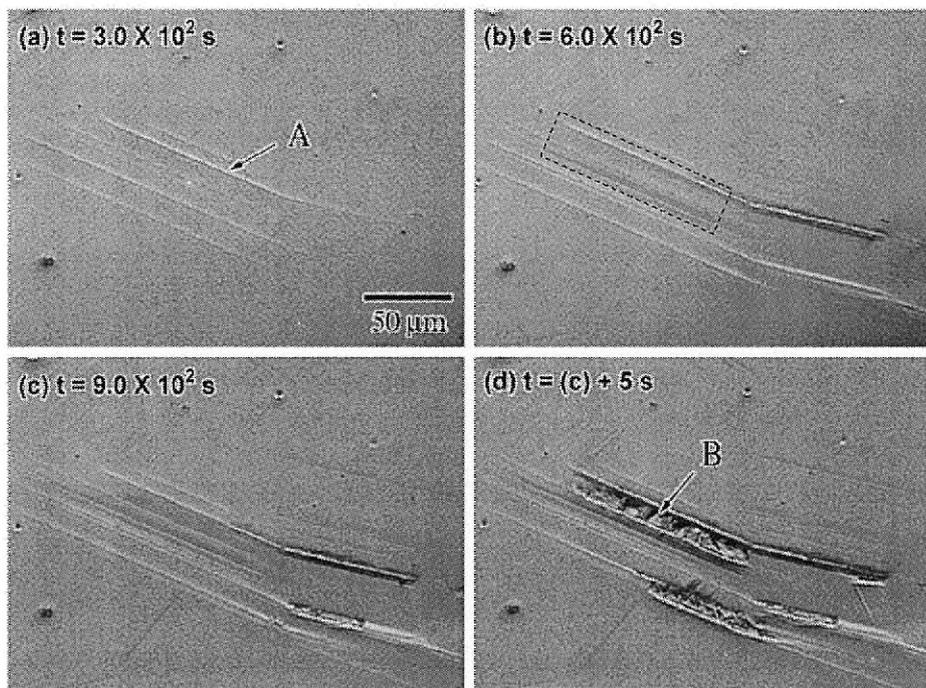
Fig. 3-6 A series of *in-situ* optical micrographs of the solution-treated SUS304L stainless steel showing successive  $\gamma \rightarrow \epsilon' \rightarrow \alpha'$  martensitic transformation at 103 K.
