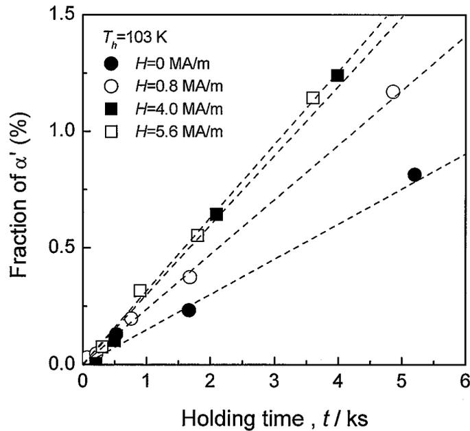
Fig. 5-2 Relation between isothermal holding time and volume fraction of  $\alpha'$ -martensite in the solution-treated SUS304L after isothermal holding at 103 K under various magnetic fields of 0, 0.8, 4.0, and 5.6 MA/m. Lines are guide for eyes.
