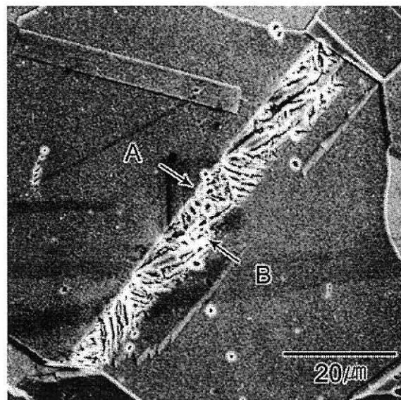
Fig. 2-4 A SEM image of a solution-treated SUS304L stainless steel after isothermal holding at 77 K for  $10^6$  s. The mark 'A' indicates a plate of  $\epsilon'$ -martensite and the mark 'B' indicates a wedge-shaped plate of  $\alpha'$ -martensite inside the  $\epsilon'$ -martensite.
