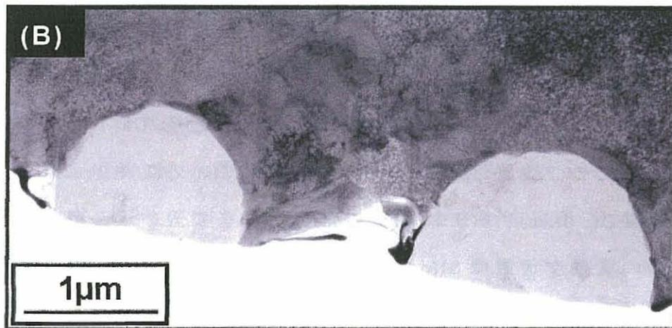
Fig.4-1 (A) is scanning ion microscopy (SIM) image of acicular ferrite in Al/O ratio of 0.73 and (B) is bright field image of the travel section of same inclusions as (A)
