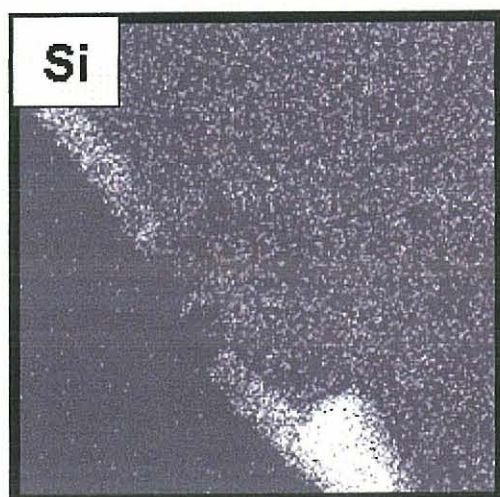
Fig.4-9 EDS mapping analyses at inclusion in Y2 (Al/O=0.73, as-welded)
