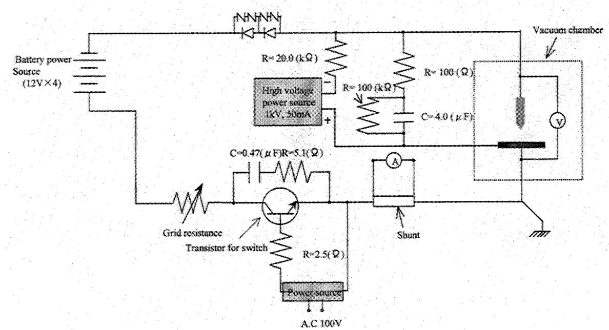
Fig.2.3 Experimental apparatus for HCA
