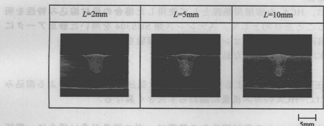
Fig.3.15 Effect of arc length on bead cross section in HCA welding:
