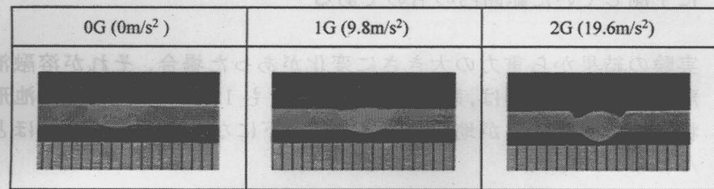
Fig.7.13 Effect of gravity on weld bead profile (Bead cross section)
