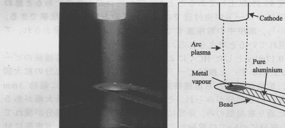
Fig.6.1 Photograph and schematic diagram of HCA on aluminium plate:
