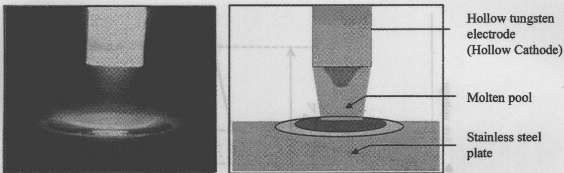
Fig.2.12 Photograph and schematic diagram of HCA.
