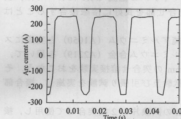
(b) Waveform of arc current
