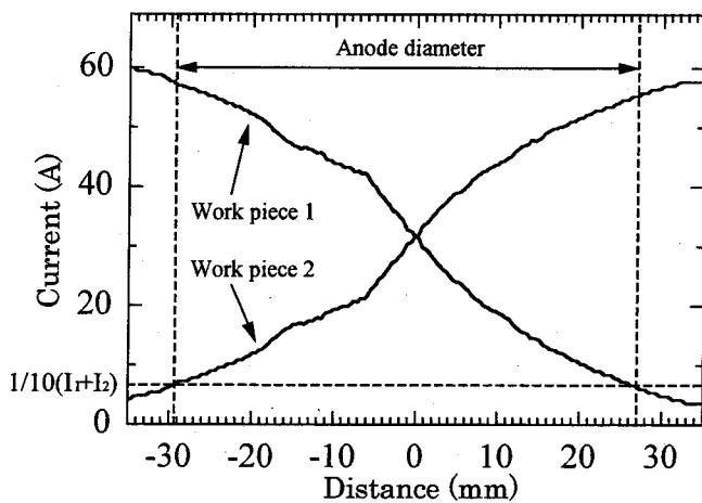
Fig.5.3 Typical example of current distribution measured by split anode method for HCA:
