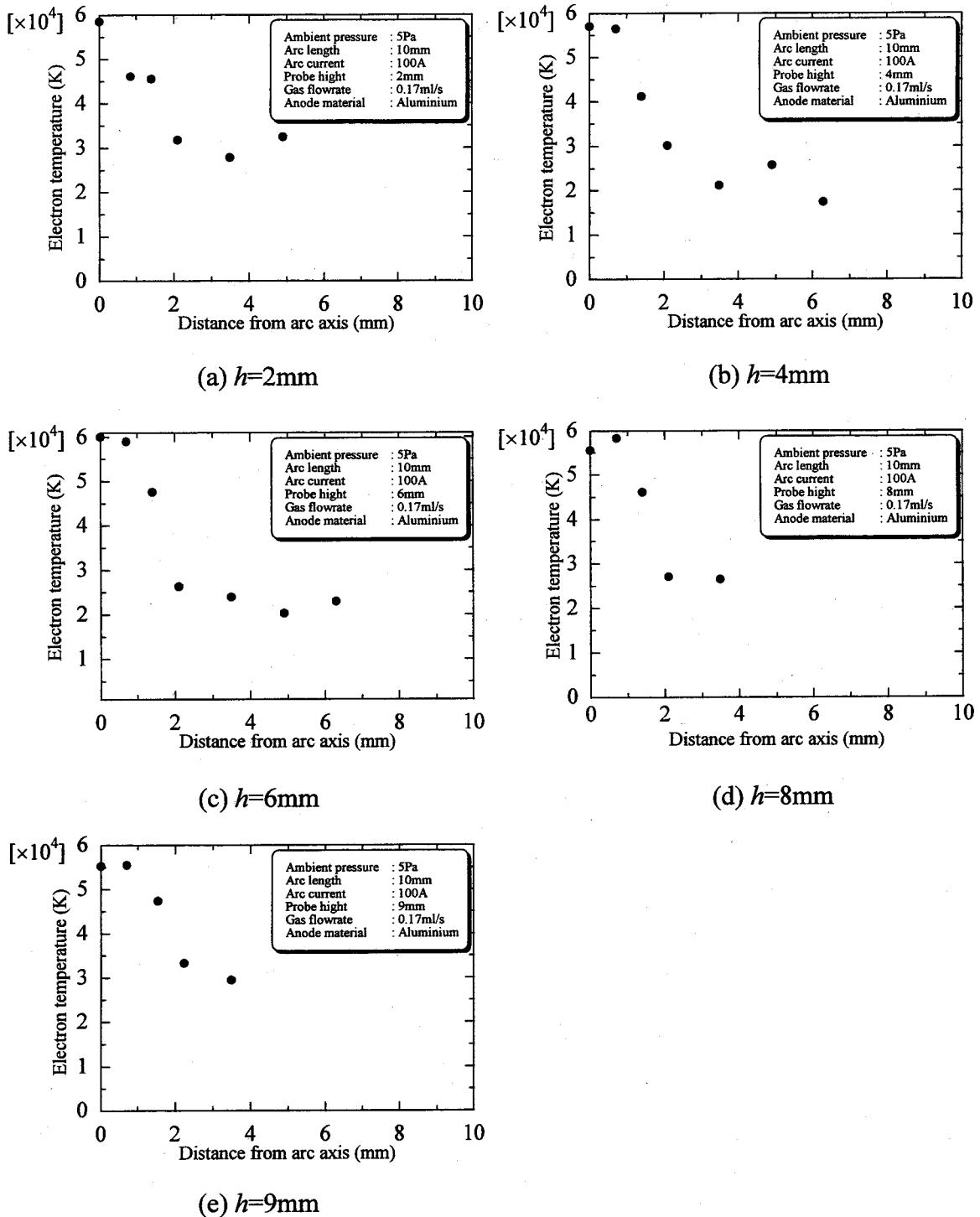
Fig.6.5 Electron temperature distribution in HCA column:
