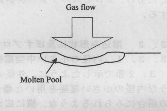
Fig.3.5 Effect of gas flow on penetration in HCA melting
