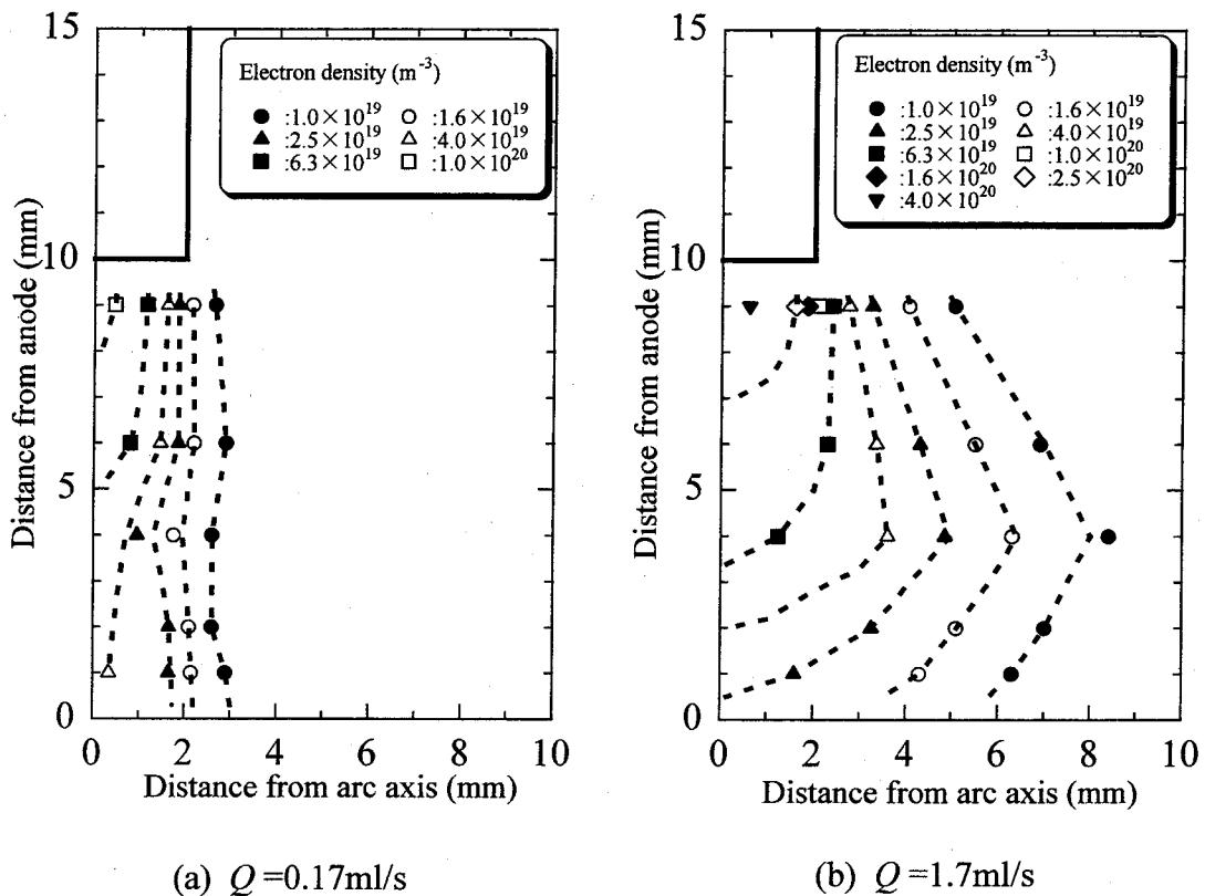
Fig.4.6 Electron density distribution between electrodes:
