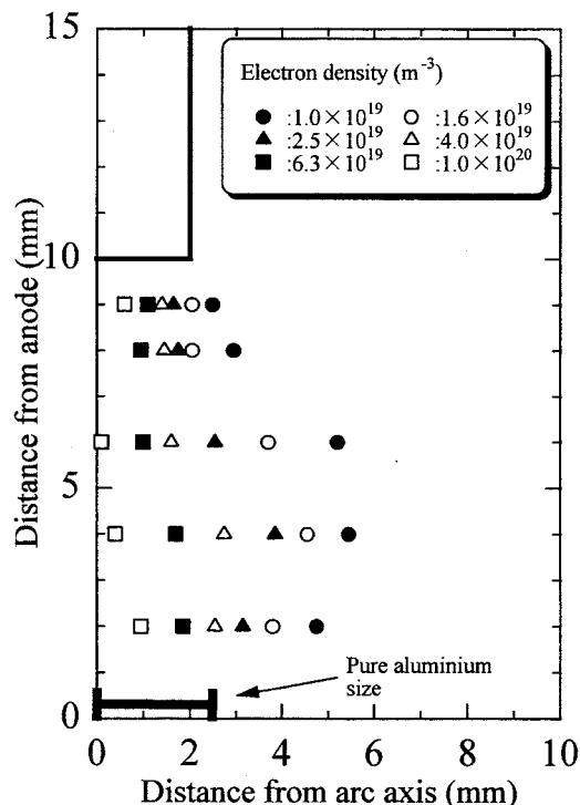
Fig.6.4 Electron density distribution between electrodes:
