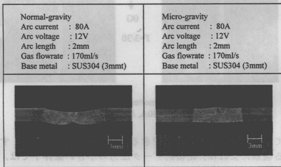
Fig.7.12 Effect of gravity on weld bead profile
