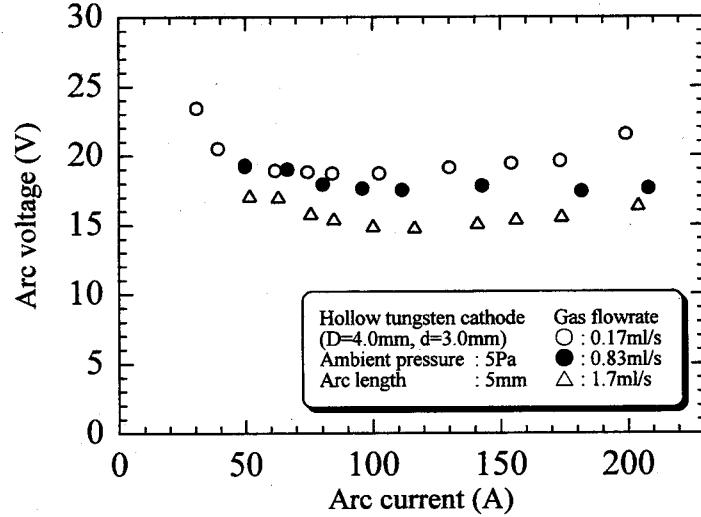
Fig.2.16 Effect of gas flowrate on arc characteristics
