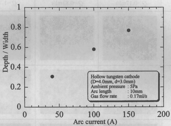
Fig.3.11 Effect of arc current on D/W rate
