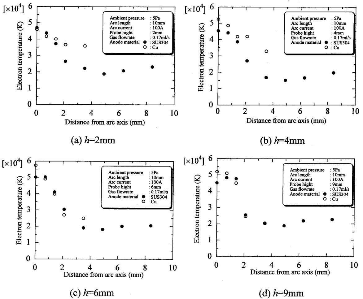
Fig.4.11 Electron temperature distribution in HCA column:
