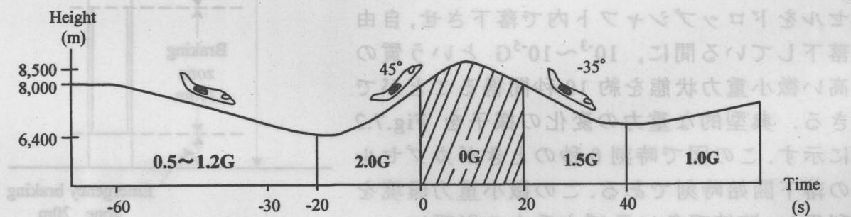
Fig.7.4 Image of parabolic flight pattern
