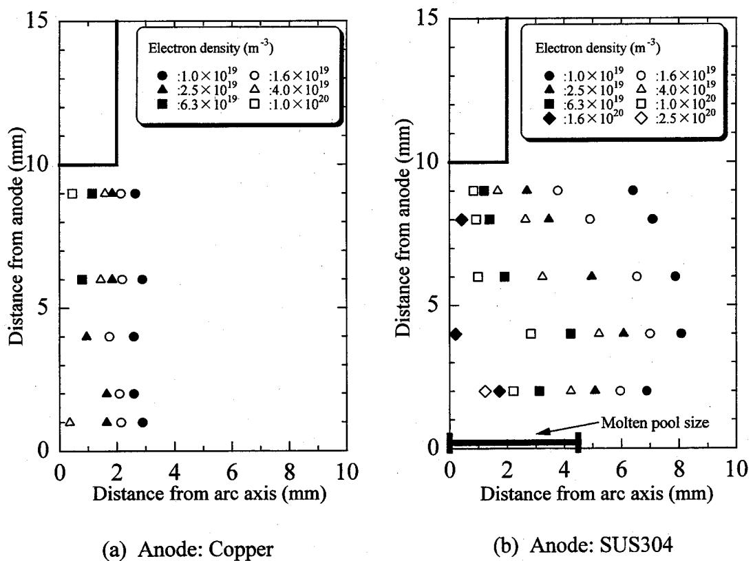
Fig.4.10 Electron density distribution between electrodes:
