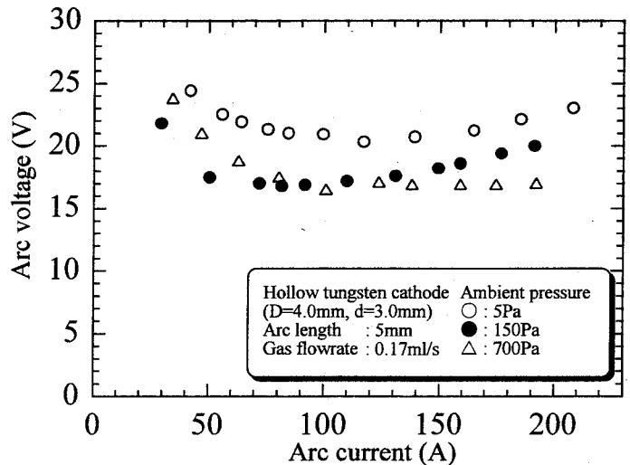
Fig.2.18 Effect of ambient pressure on arc characteristics
