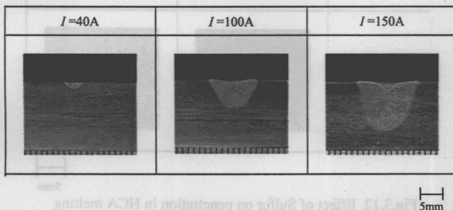
Fig.3.10 Effect of arc current on penetration in HCA melting:
