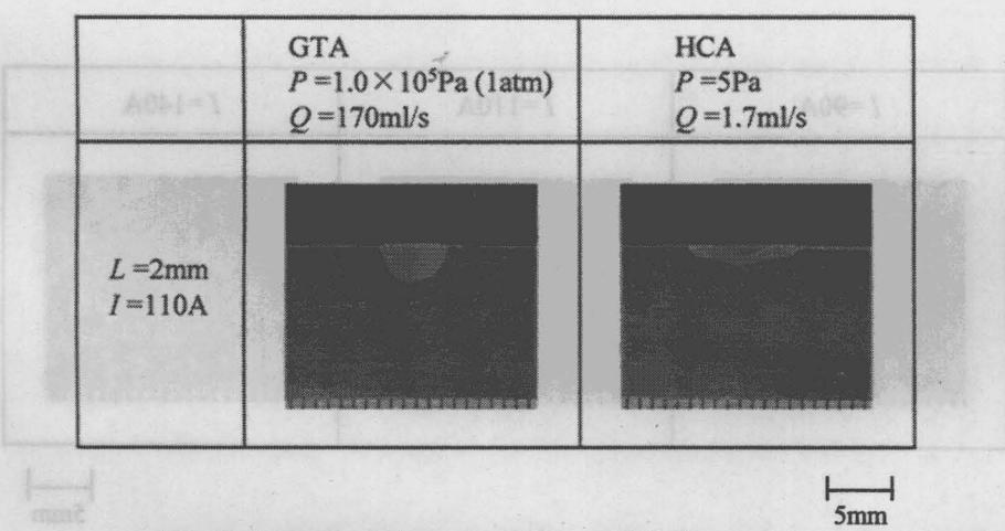
Fig.3.4 Penetrations in GTA and HCA melting
