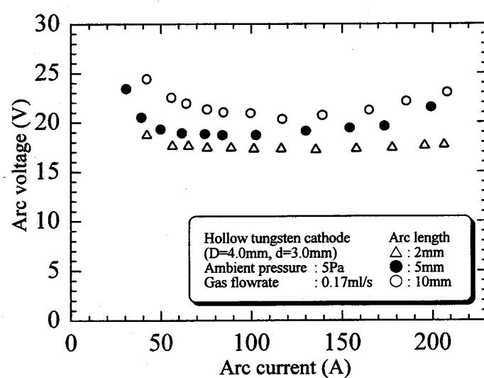
Fig.2.17 Effect of arc length on arc characteristics
