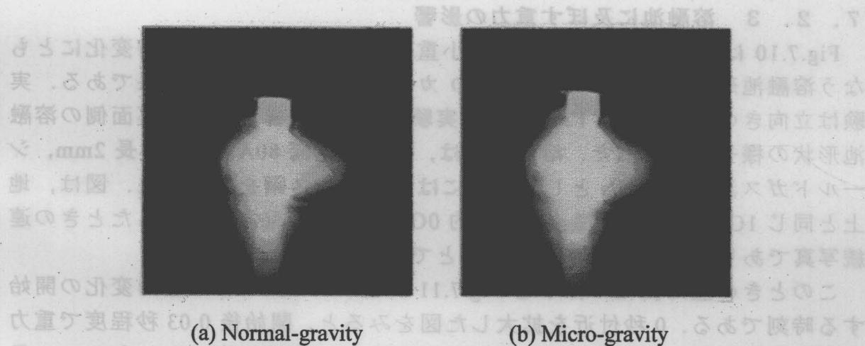
Fig.7.8 Appearance of GTA in welding
