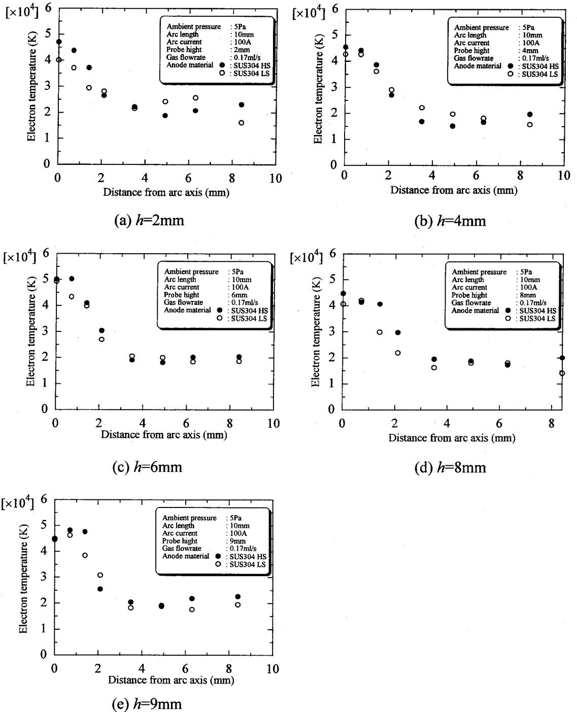
Fig.4.13 Electron temperature distribution in HCA column:
