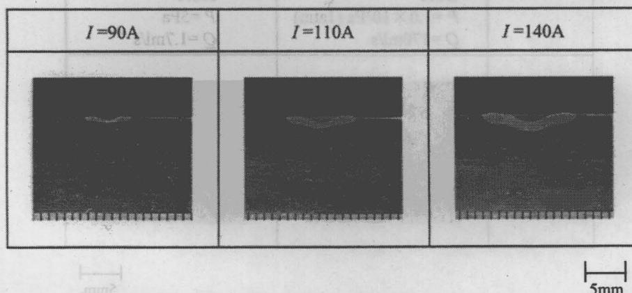
Fig.3.6 Effect of arc current on penetration in HCA melting:
