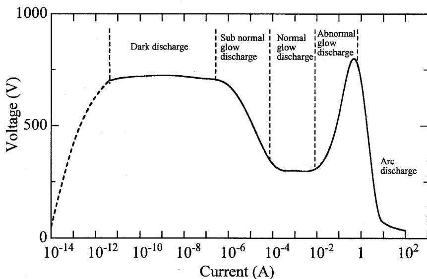
Fig.2.4 Discharge characteristics of gas
