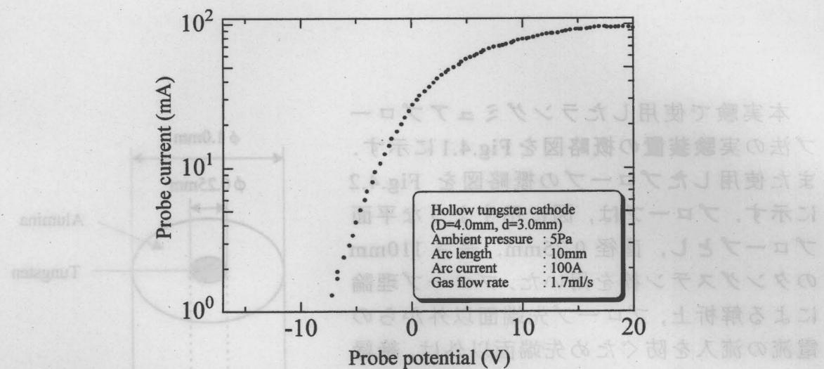
Fig.4.4 Example of Langmuir probe characteristic for HCA plasma
