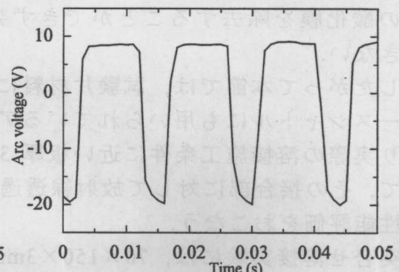
(c) Waveform of arc voltage
