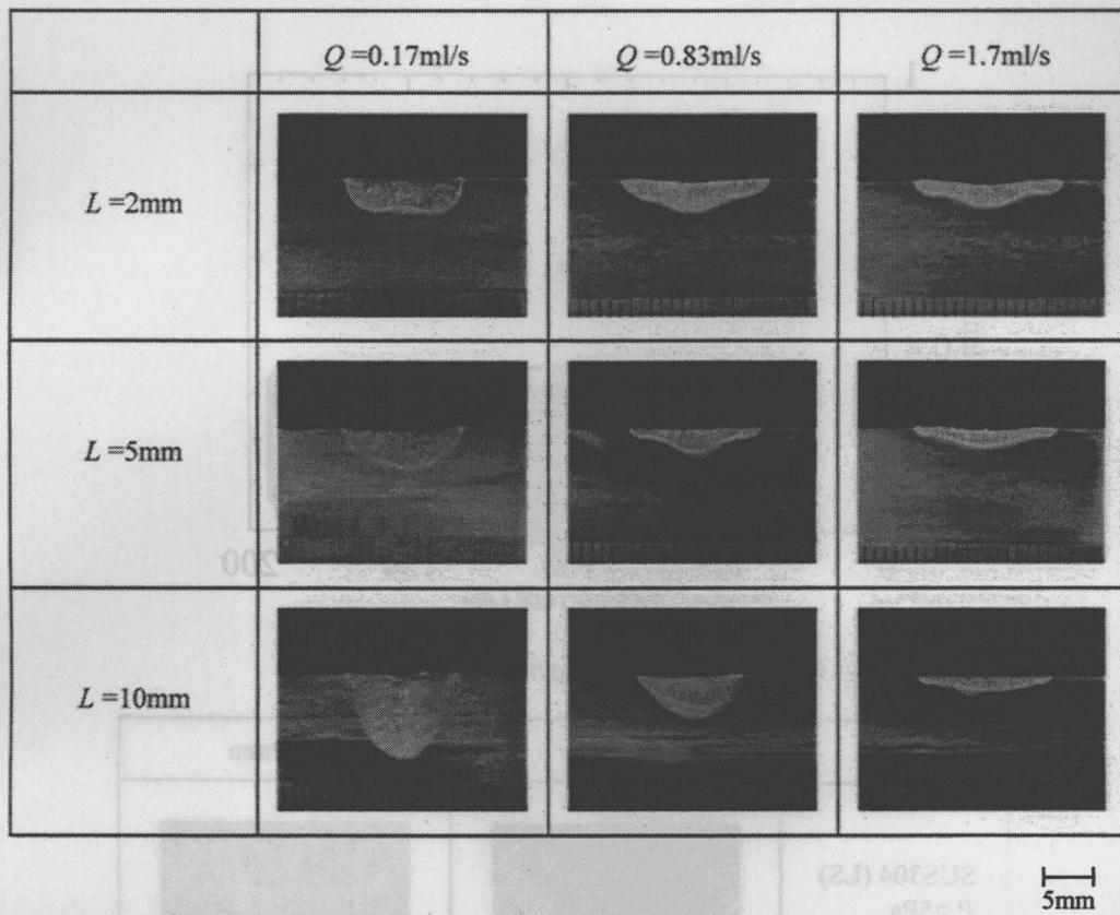
Fig.3.9 Effect of arc length and gas flow rate on penetration in HCA melting
