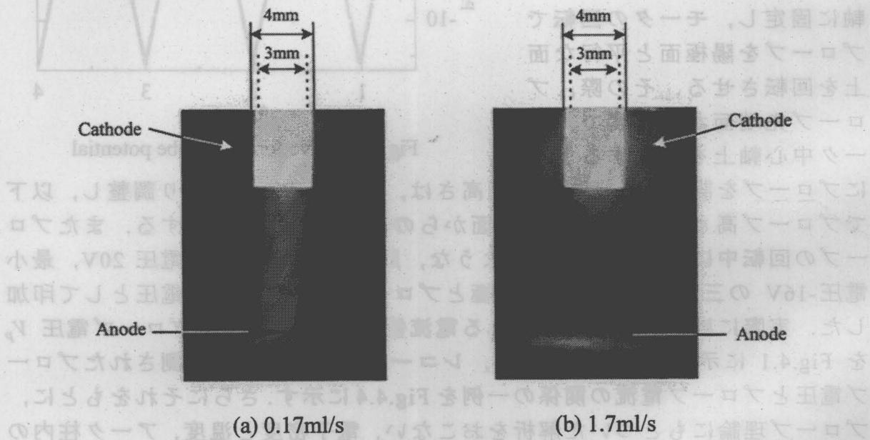
Fig.4.5 HCA discharge measured by probe method
