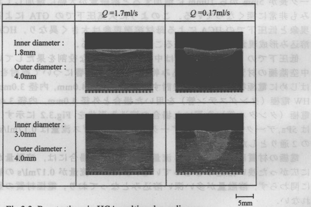
Fig.3.3 Penetrations in HCA melting depending on electrode inner diameter:
