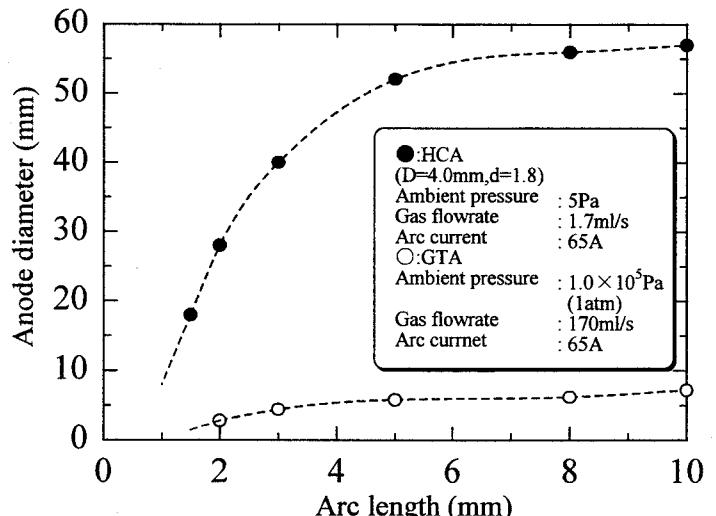
Fig.5.4 Comparison of anode diameters between HCA and GTA
