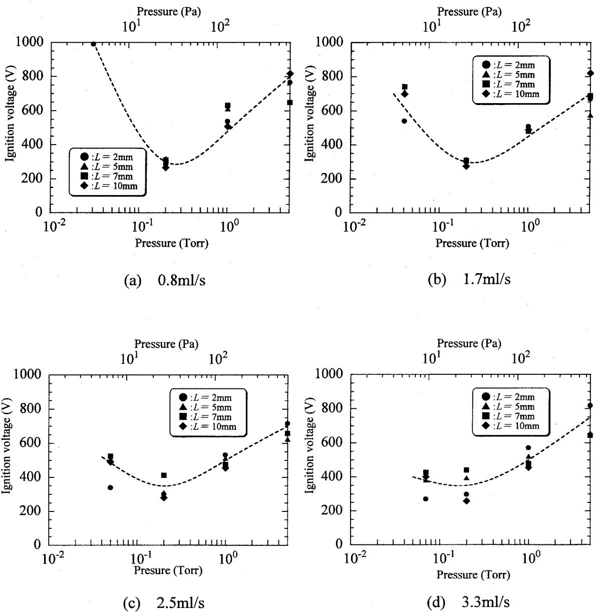
Fig.2.6 Relationship between ambient pressure and ignition voltage
