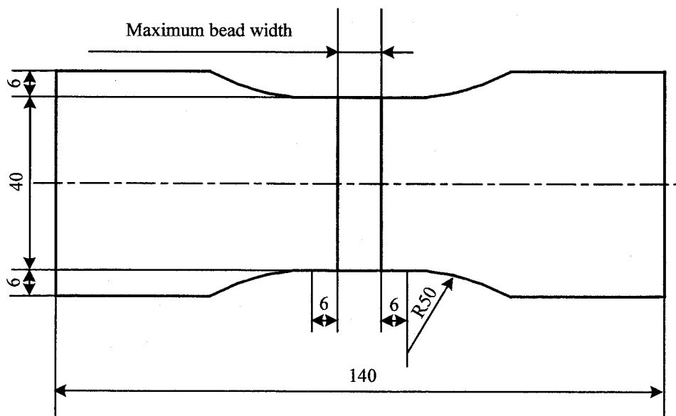
Fig.6.11 Size of test piece for tensile test
