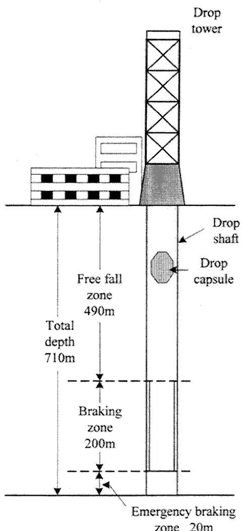
Fig.7.1 Schematic of the Japan Microgravity Center (JAMIC)
