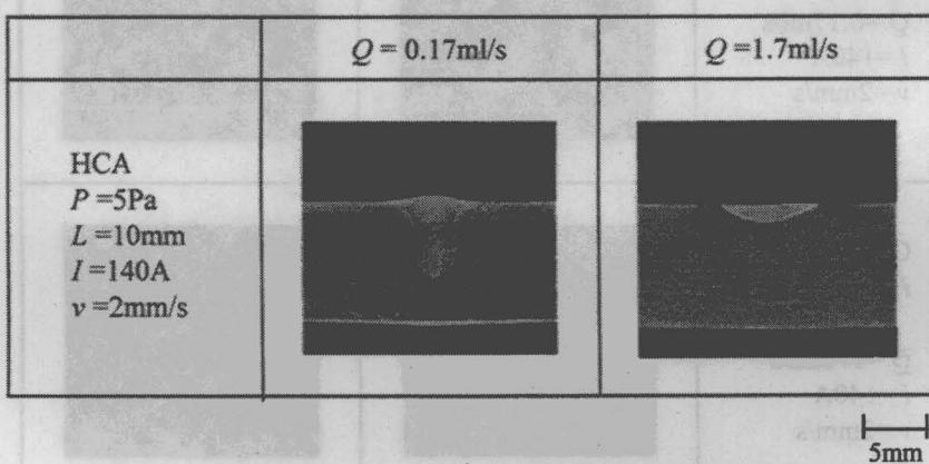
Fig.3.14 Effect of gas flowrate on bead cross section in HCA welding: ambient pressure 5Pa, arc current 140A, arc length 10mm, welding speed 2mm/s hollow tungsten cathode ( $D = 4.0\text{mm}$ ,  $d = 3.0\text{mm}$ )
